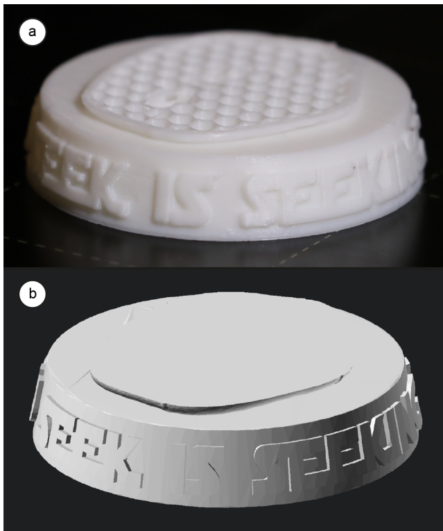
Figure 3: Comparison between the result of a failed 3D print and the geometry created by our generator: (a) A 3D print that failed mid-fabrication. (b) The mesh generated of our failed print generator.
