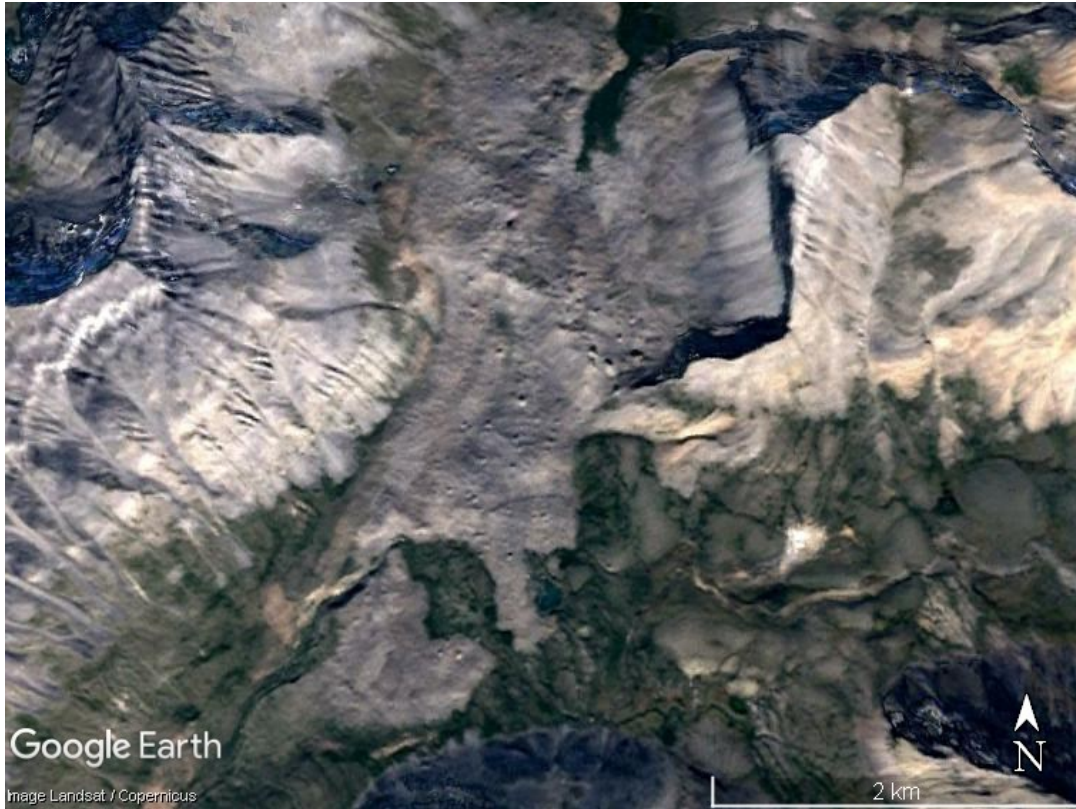
Figure 2.1 Rockslide Pass in the Mackenzie Mountains is a large rock avalanche with a volume of 450 Mm 3 and travelled about 4.4 km, it is one of the largest rock avalanches to have occurred in the Canadian Cordillera area (Eisbacher, 1979; Google Earth, 2021c).
