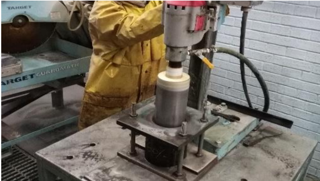
Figure 3-6 Coring a Cylindrical Asphalt Specimen (Al-Bayati, 2019)
