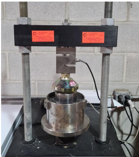
c. Loading Frame
