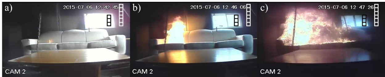
Figure 3.25: Cam2 light (black outline) and dark (white outline) areas at a) 35 seconds (reference image) b) 240 seconds and c) 320 seconds [85]
