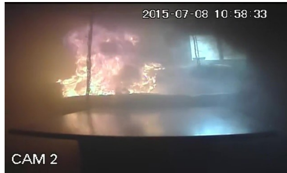
Figure 4.24: Fire proximity impact on smoke layer visible in angle of smoke layer over window
