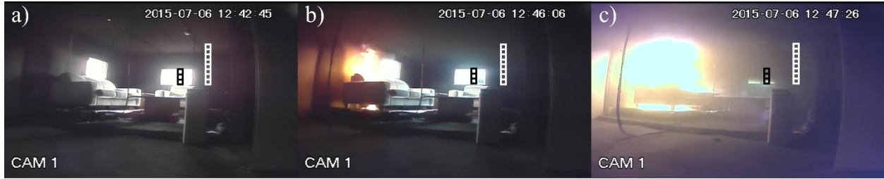
Figure 3.22: Cam1 light (black outline) and dark (white outline) areas at a) 35 seconds (reference image) b) 240 seconds and c) 320 seconds [85]
