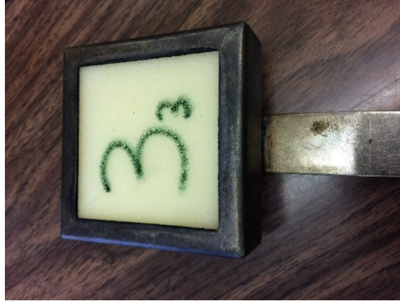
Figure 2.8: Smoke density chamber ISO 5659-2 sample holder with a sample of material 3 (flexible polyurethane foam) for the third repetition in a particular heating mode
