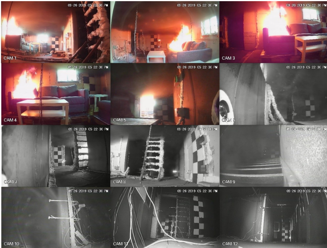
Figure 3.8: Time-synchronized images from cameras with interior views (V1-12) 210 seconds after ignition in experiment F1
