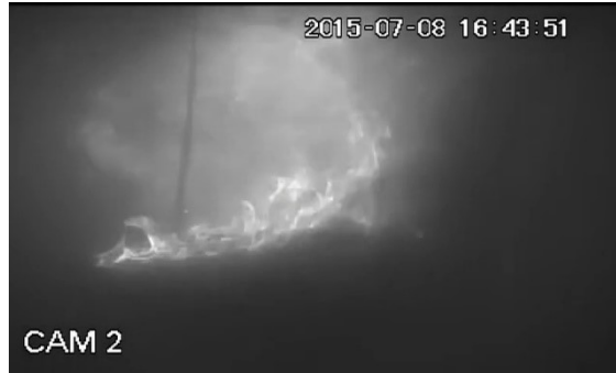
Figure 4.1: Cam2 Image 360 s after crib ignition in experiment A2 (time of Cam1 obscuration)
