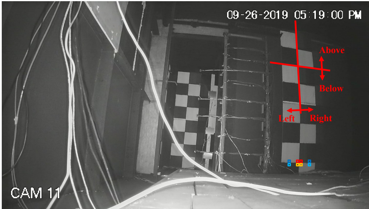
Figure 4.33: Position influence of lighting on radiance values for experiment F1 camera V11 and checkerboard CB11A
