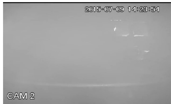
Figure 4.2: Cam2 Image 1140 s after crib ignition in experiment C2 (shortly before obscuration)
