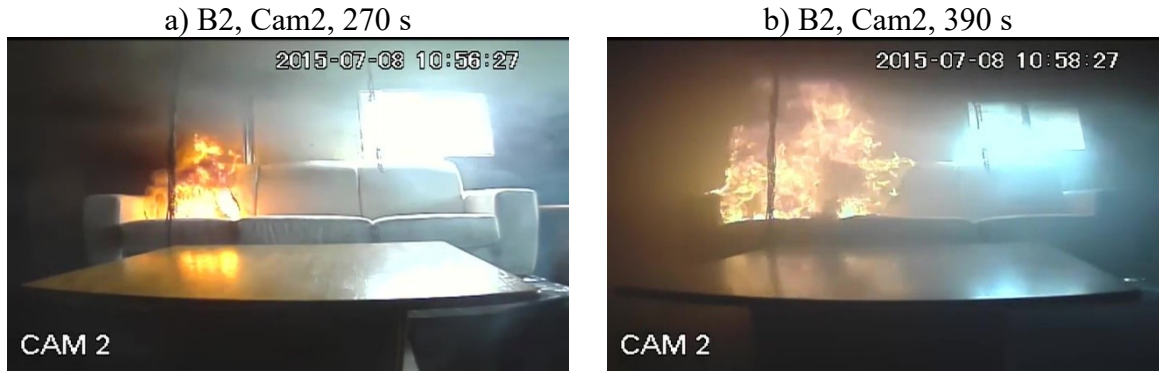
Figure 4.4: Experiment B2 Cam2 images with a) a “thin” smoke layer visible 270 s and b) the “bulk” of the smoke layer visible at 390 s after crib ignition
