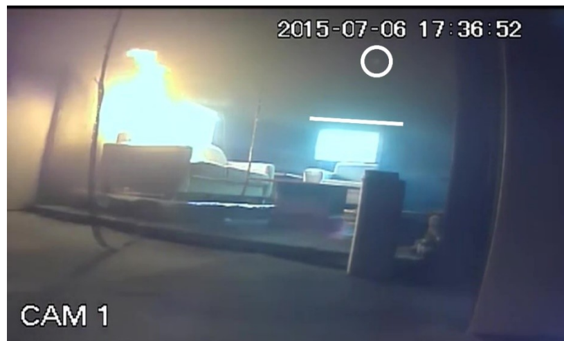
Figure 4.14: Cam1 image from 480 s after ignition in experiment C1 showing the smoke detector (circled) almost entirely obscured and the smoke layer above the window (underlined)
