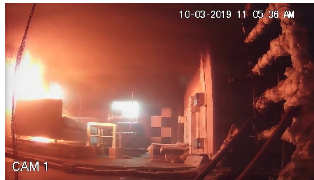
Figure 4.36: Experiment F2 at 270 s showing the smoke layer appearing lower on the checkerboard than the window
