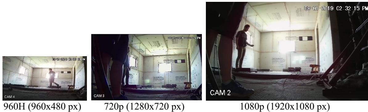
Figure 3.7: Representative images for the V1 and CB1 location at 960H (left), 720p (middle) and 1080p (right) resolutions displayed at 15% of their original size.
