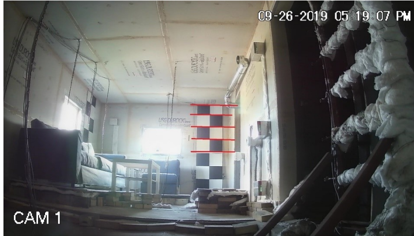
Figure 4.56: Observers estimated smoke layer descent time to each of the five heights ( z=2.30 m, 2.07 m, 1.77 m, 1.46 m, 1.16 m) indicated with red lines on checkerboard CB1 from camera V1
