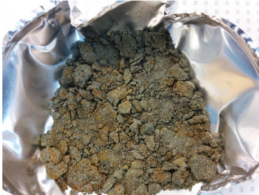
Figure S5.3: Photo of tailings samples collected from the upper part (from 1.18 to 1.36 m bgs) of the paleo-oxidized layer.
