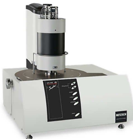
Figure 3.3 DSC/TGA measurement and analysis system [26]
