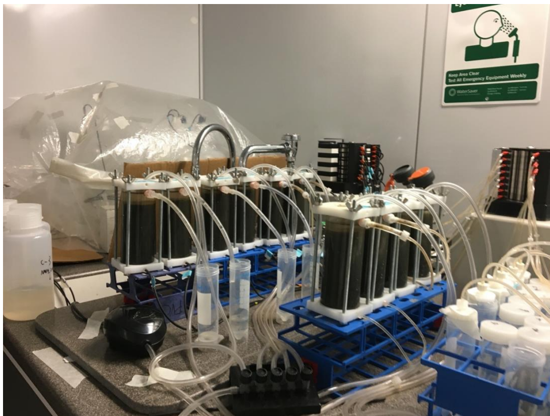
Figure 5.1. Diagram of the flow-through column system (top) and a photo of the experimental set-up (bottom). Illustrated in the top diagram, from left to right of: deoxygenated influent reservoir with a Tedlar bag (5 L, Millipore Sigma) filled with pure N_2 , a peristaltic pump for maintaining the flow rate of 5 \text{ mL h}^{-1} , the sediment column with overlying water and a top plate with openings that remain open during oxic periods and are closed under anoxic conditions, a falcon tube for sampling the outflow of overlying water, and compressed air to keep overlying water well oxygenated (during oxic periods).
