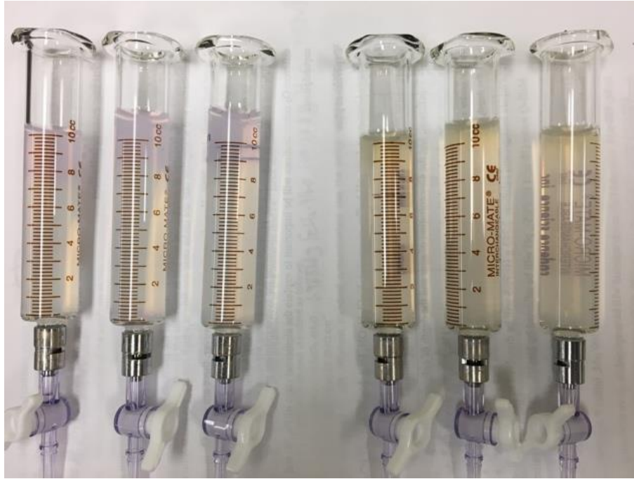
Figure 4.2. Photo of agarose column experiment. 1% agarose (wt. %) was melted under anoxic conditions, Fe(II) was added to the solution for the three columns pictured on the right, and the solution was allocated to 10 mL metal male luer-lock glass syringes to solidify in the anaerobic chamber. After the solidification of the agarose, columns were taken out of the chamber and exposed to air at one end. This photo was taken after 6 hours of exposing the columns to air at 25 \pm 1 °C. The three columns shown on the left contain background solution with sodium resazurin to show the diffusion of oxygen (Uzarski et al., 2017). The diffusion of oxygen in these columns is evident by the blue-purple colour that can be seen in the near-surface agarose. The three columns shown on the right contain about 300 \mu\text{M} initial Fe(II) concentration in their background solution.
