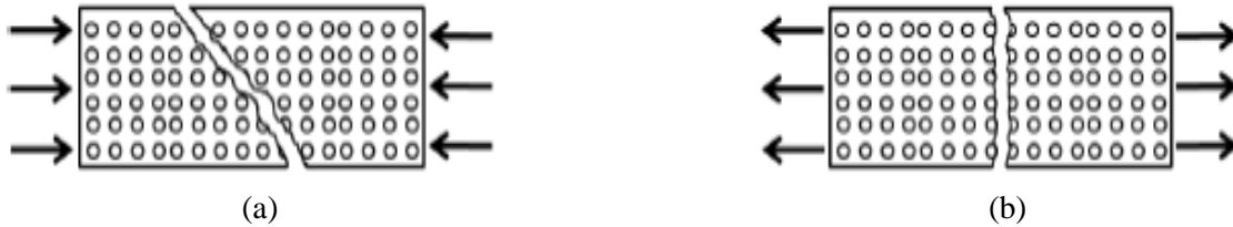
Figure 9. Matrix failure mode for a UD lamina: (a) transverse compression, and (b) transverse tension.
