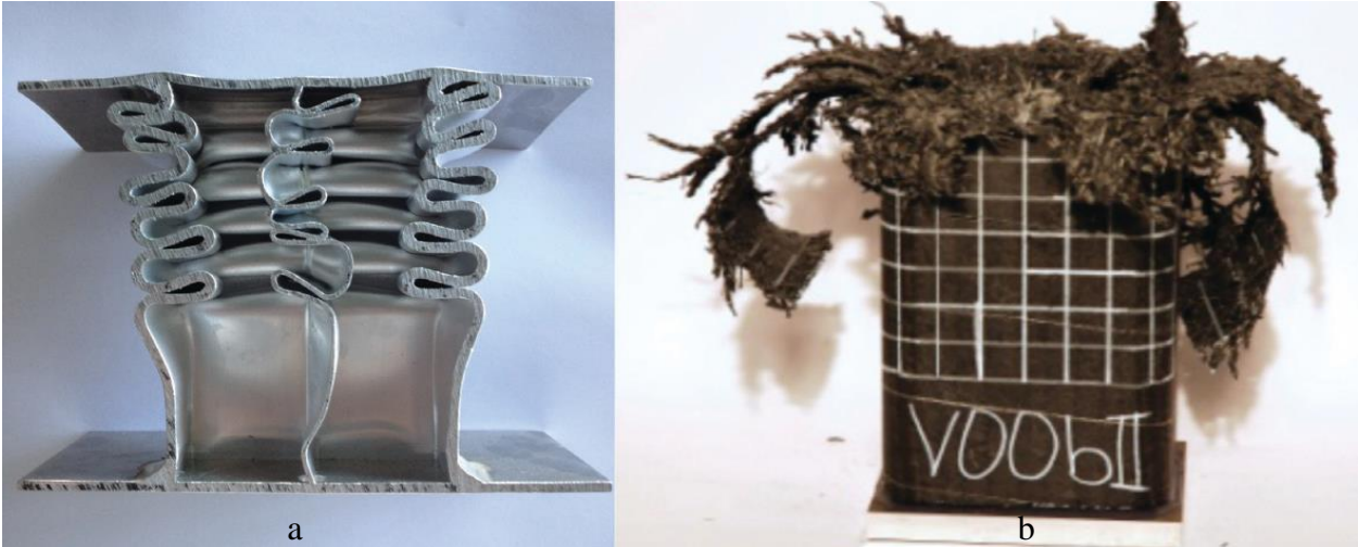
Figure 17 Comparison of metals and FRP composites under axial crush load: (a) plastic folding in metal component, and (b) brittle fragmentation in an FRP component [66].
