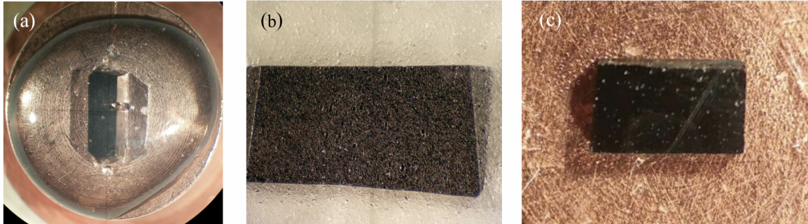
Figure 4.8: Surfaces after sample polishing techniques with a micro grit paper and a granite slab assembly in our lab. Details discussed in the text.
