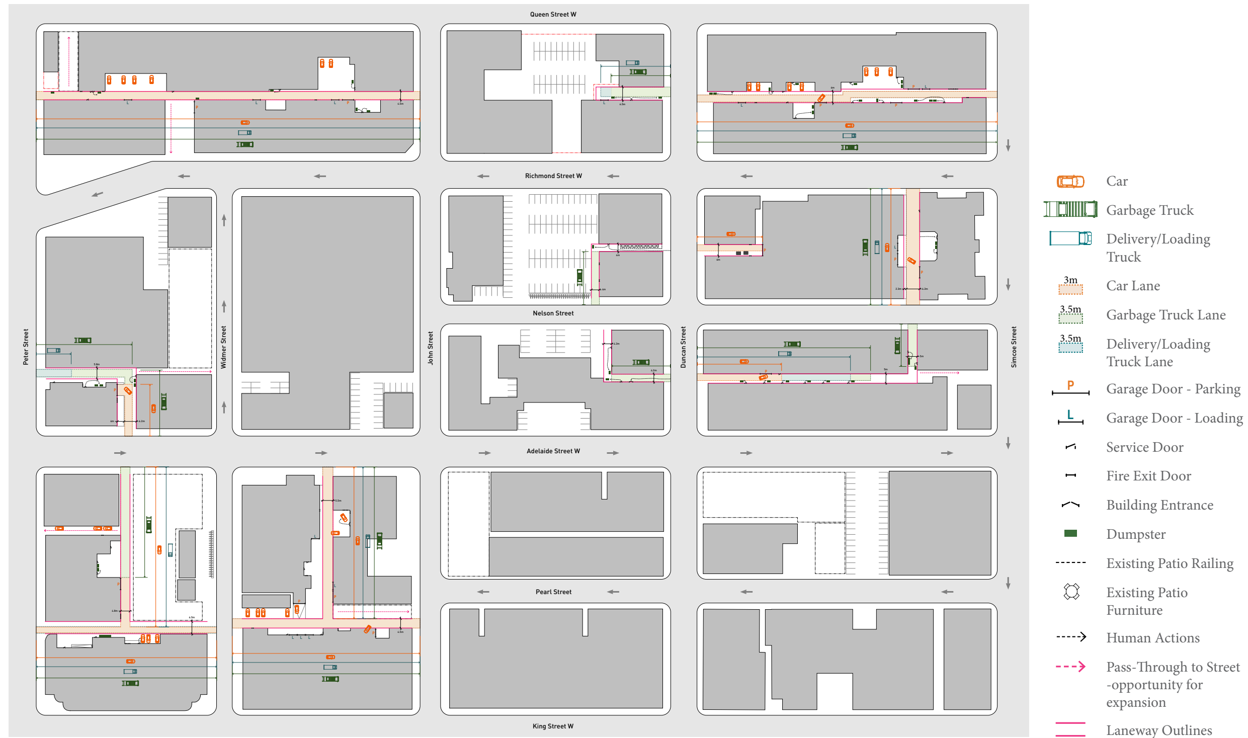
Fig. 155 - Existing Service Conditions; Overall Network, plan
