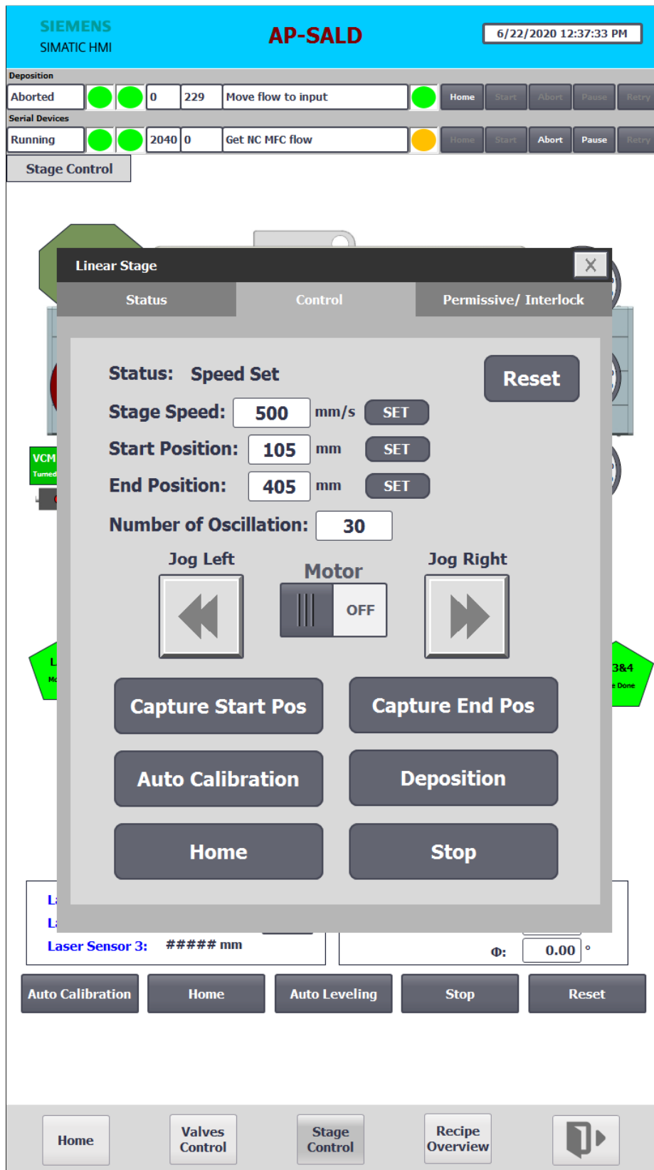
Figure A.18 The linear stage's control interface of HMI.
