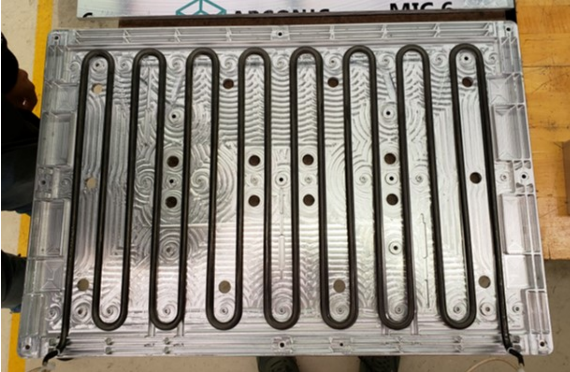
Figure 2.22 A picture of the customized heating element.
