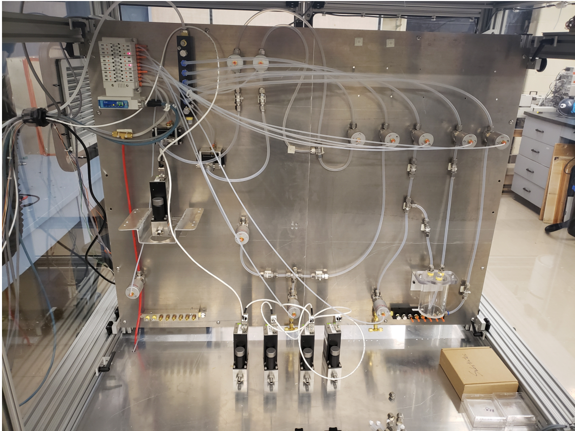
Figure 3.12 MFCs were dismantled from the bubbling panel for the leak test.
