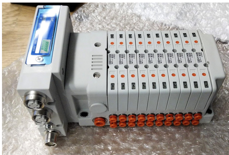
Figure 2.6 A picture of SMC SS0750 pneumatic manifold with EX260 serial transmission system.
