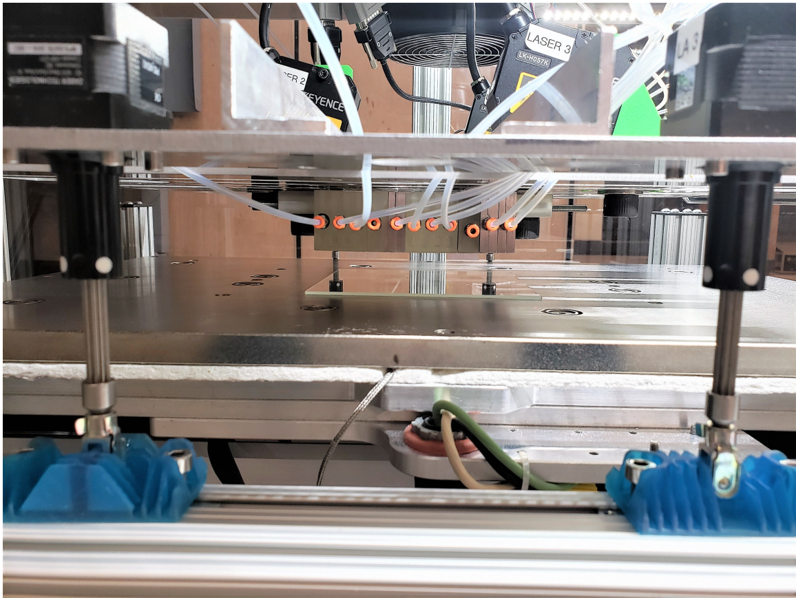
Figure 2.19 The actual setup of the reactor head with linear actuators and laser sensors.
