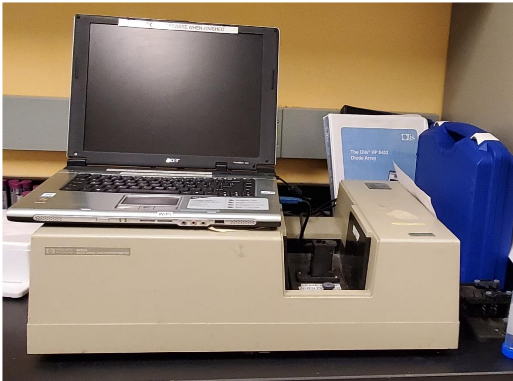
Figure 2.17: HP 8452 Diode Array Spectrophotometer used to measure the absorption spectrum of ozone and the anesthetic gases
