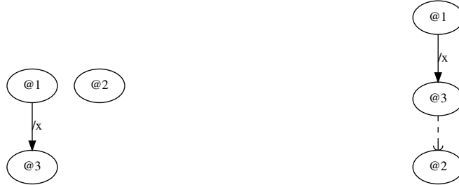
(a) The initial environment with three values @1, @2 and @3 and a field x (b) The environment with @3 and @2 merged, preserving @2
