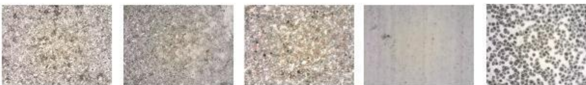
Figure 3. 5: Microscopic images (200x) of test surfaces post immersion in artificial ocean water
