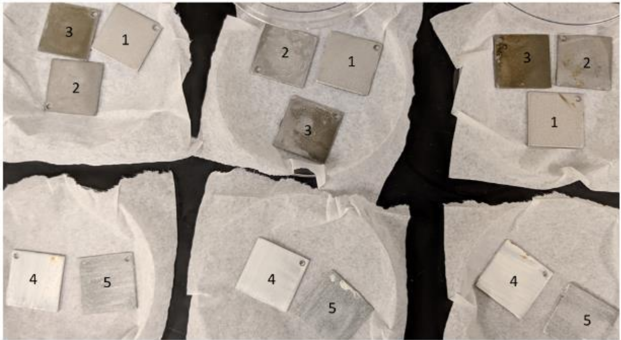
Figure 3. 11: Samples immersed in different concentrations (1%, 10% and 30%) of hydrogen peroxide for 24 hours
