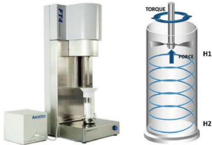
Figure 3.2 The FT4 powder rheometer system and the flow pattern that its blade create [102]
