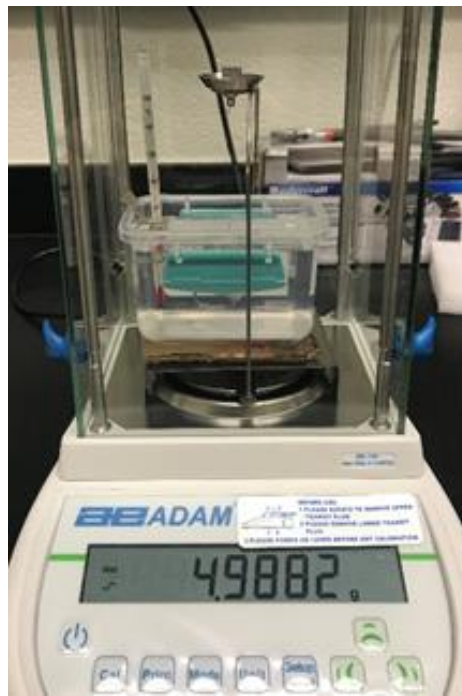
Figure 3.9 Archimedes setup for density measurement of sintered samples
