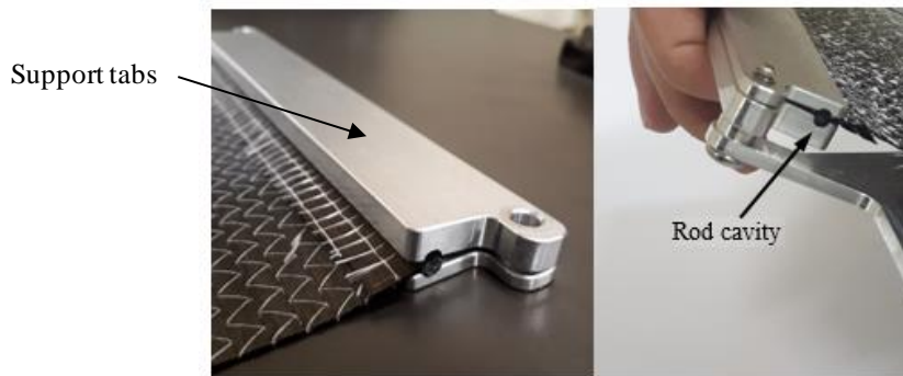
Figure 3.9. Images of the custom PFT fixture clamping mechanism illustrating the wrapped fabric specimen ends around an acrylic rod inserted into the cavity of the support tabs.
