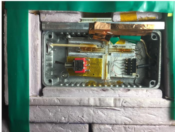
Figure 2.2: Picture of the Hall measurement sample holder box and the sample holder.
