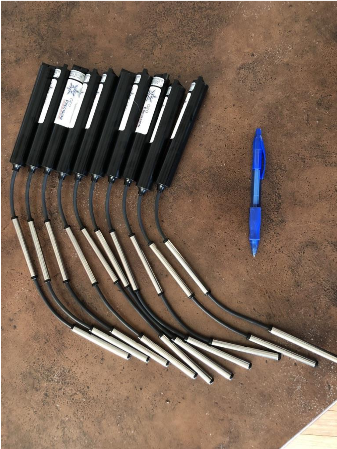
GeoPrecision thermistor strings prior to installation. Taken January 16, 2019.
