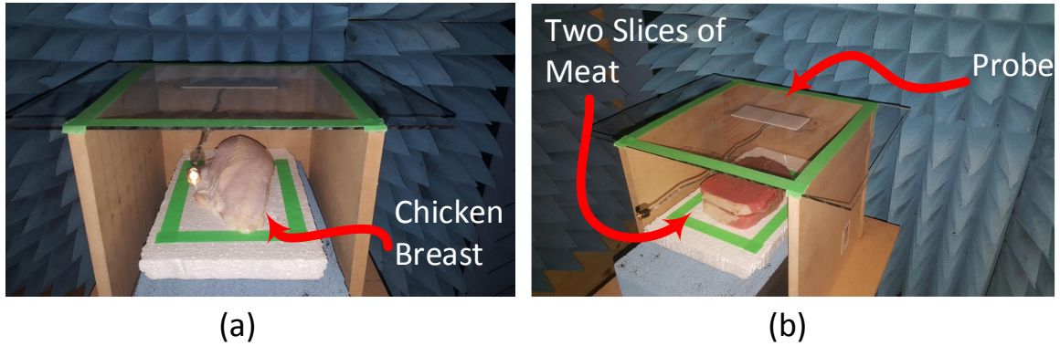
Figure 3.5: Experiment setup: (a) The ultra-narrow band probe with chicken breast. (b) The ultra-narrow band probe with two slice of meat.
