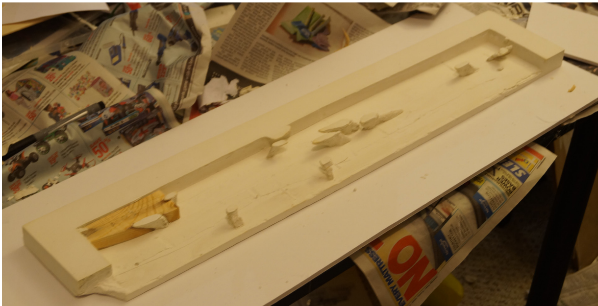
Figure 2.20 - SPF progress photos 8 - The end result of one half of the mold showing the casts of the beetle trails.
