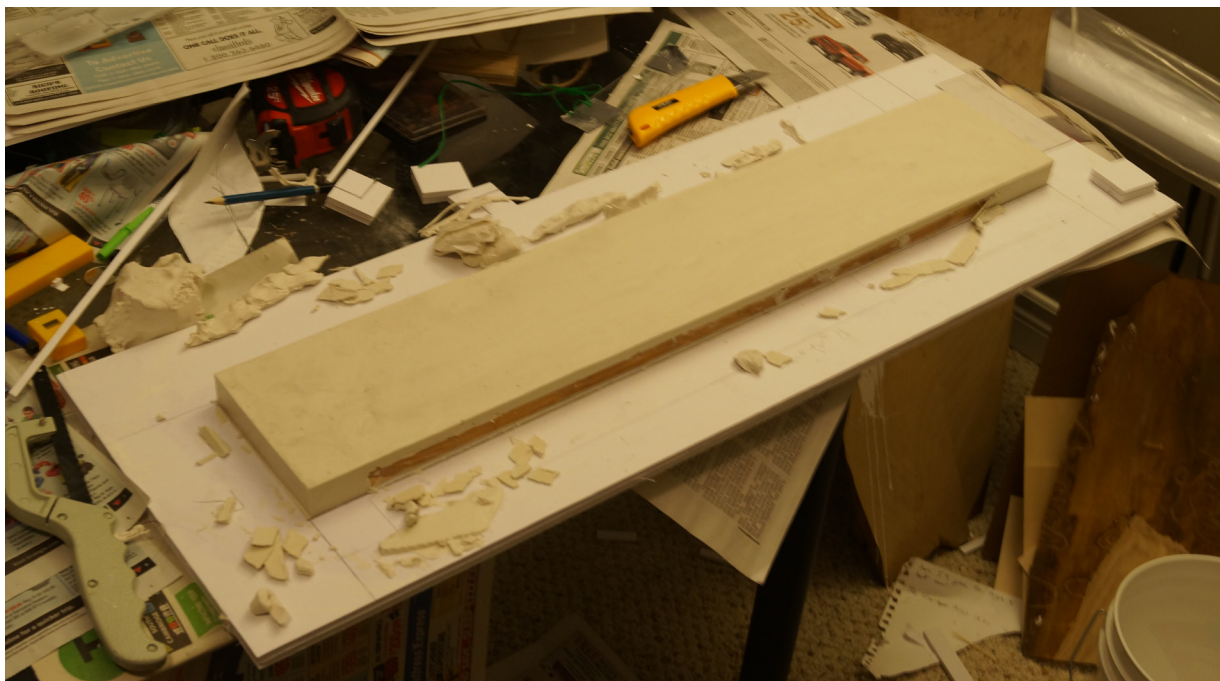
Figure 2.18 - SPF progress photos 6 - Wanting to make sure that the plaster could flow into the beetle trails, I made a watery plaster of Paris mixture, but this did take an extremely long time to set.
