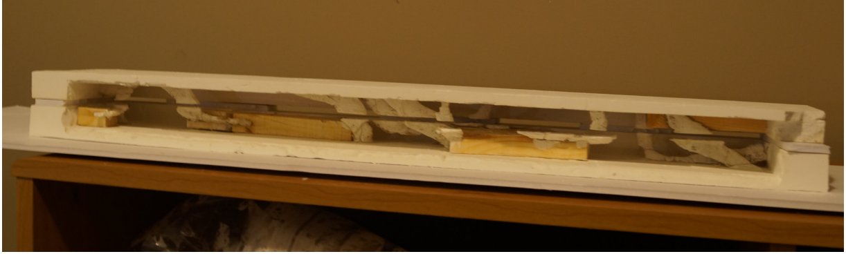
Figure 2.20 - SPF progress photos 9 - Both halves of the cast placed together after most of the wood has been removed.
