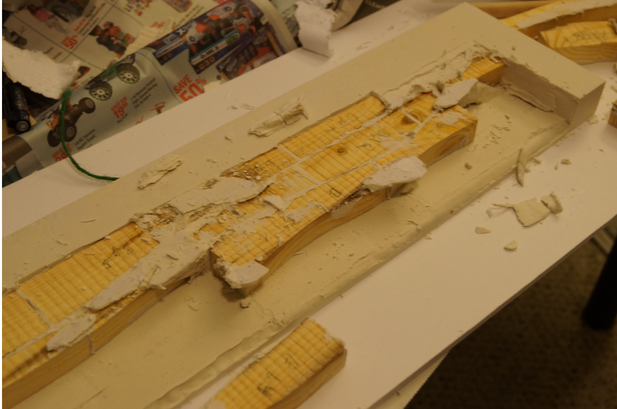
Figure 2.19 - SPF progress photos 7 - I slowly picked apart the jigsaw puzzle I had made from the wood. The Modeling clay made this a much easier process. Several of the more complex shapes were still very hard to remove requiring small wood cutting tools to cut loose.
