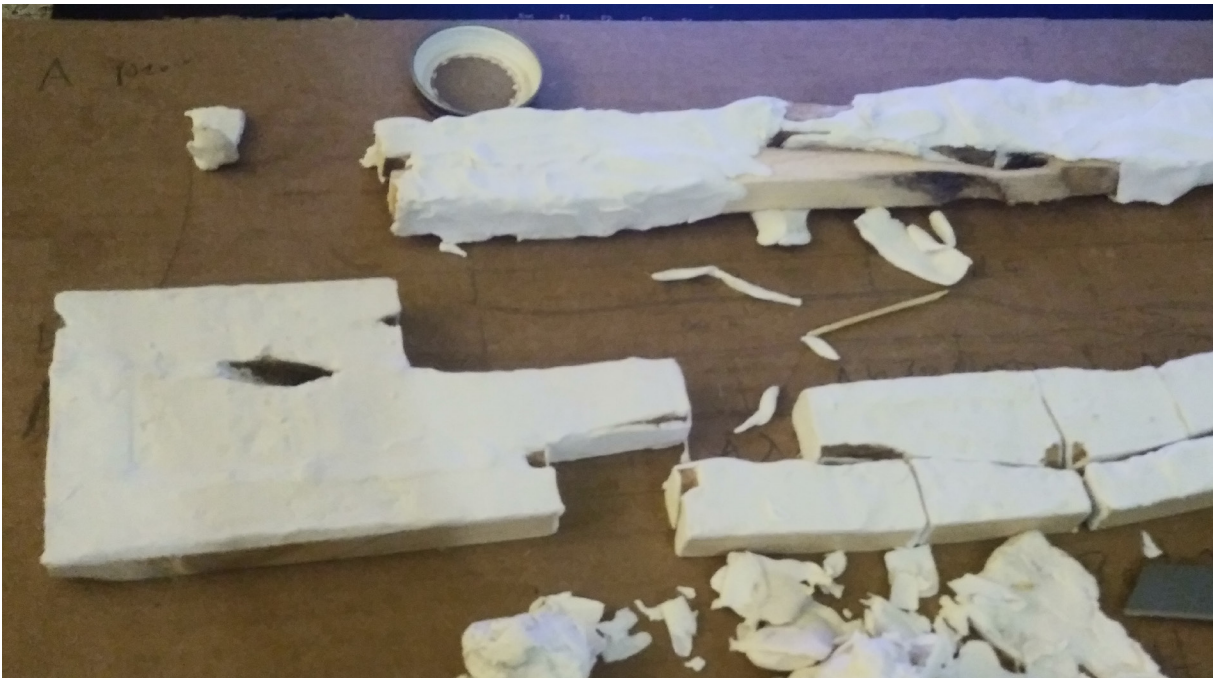
Figure 2.16 - SPF progress photos 4 - I chose to cut through the holes at 3 or 4 points where possible while filling the lost material from the cuts with modeling clay. Here I am stitching together the cut apart wood with copious amounts of modeling clay. Each piece needed to be fully covered as the modeling clay will not stick to the wood but will easily bind to itself.
