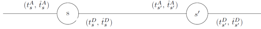
Figure 1: The general scheme of train movements at two successive stations s and s' = s + 1 . Up: nominal and actual arrivals ( A ), Down: nominal and actual departures ( D ).
