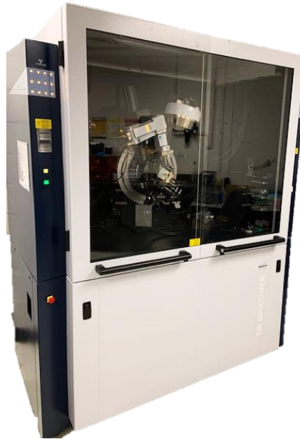
Figure 19. Bruker D8-Discover XRD machine
