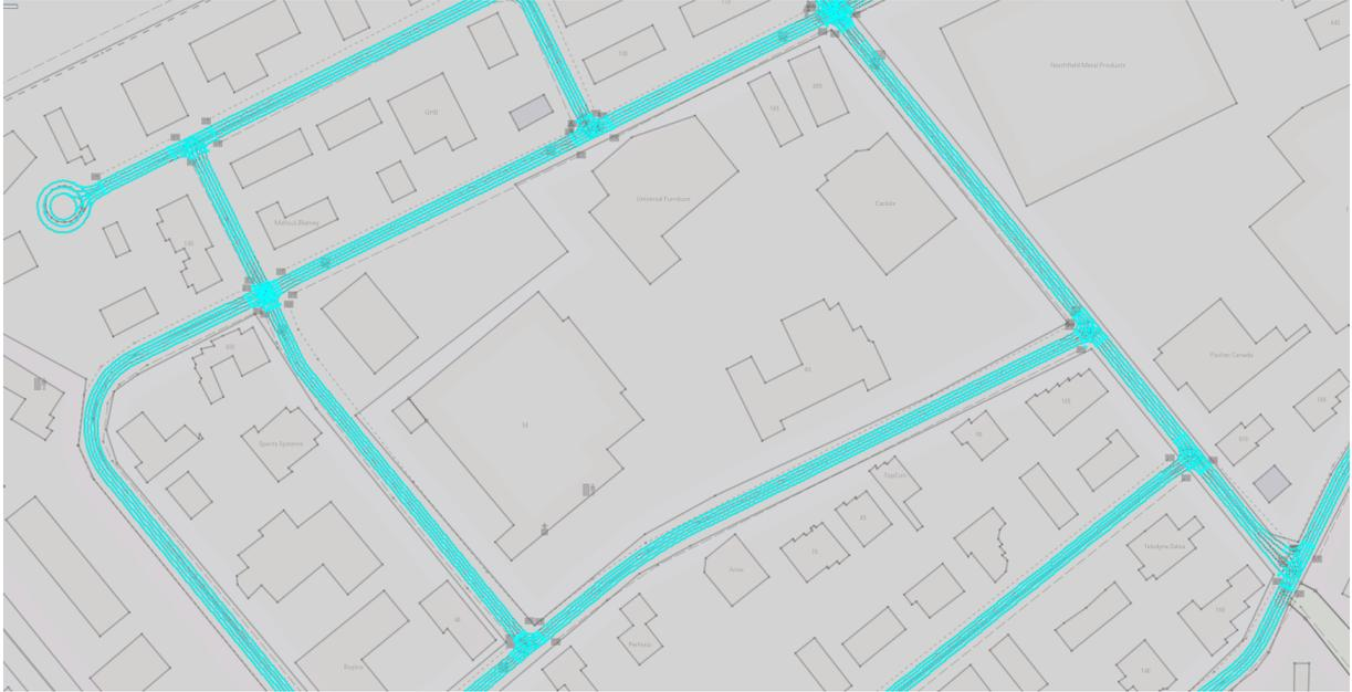
Figure 2.1: Road map constructed using lanelets (in light blue).
