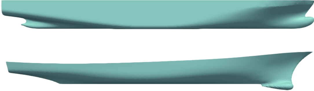
Figure 4.5: The geometry of the ship model. Top: DTC; Bottom: DTMB 5415.
