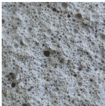
Figure 7.3.3k Vertical fracture surface was highly planar for 710kg/m 3 cem. dens., 0:1 filler-binder ratio mix. 4x magnification
