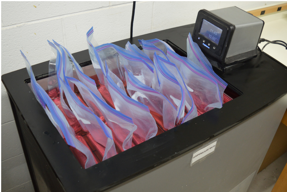
Figure 5.7.1b Specimens were suspended in a freeze-thaw bath of 30% propylene glycol, and subjected to 12 freeze-thaw cycles. Evident length change (dilation) in the sample was deemed to have been caused by freeze-thaw damage.
