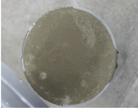
Figure 6.1.1a Bleedwater evident on surface of a freshly-cast cylinder.
