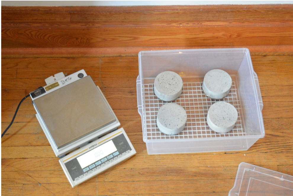
Figure 5.5.4b 100 x 50mm specimens, with lower surface immersed in 1 to 3mm of water, for capillary water uptake testing.
