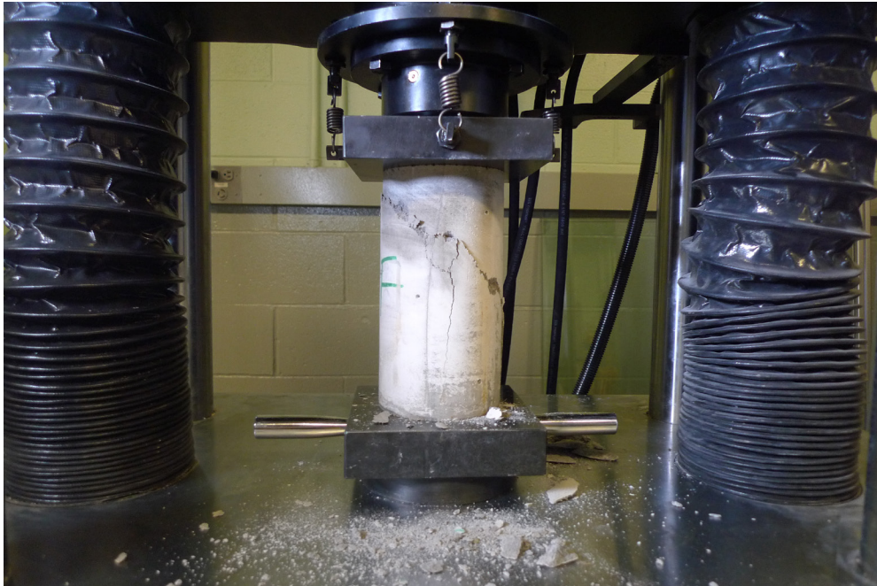
Figure 5.4.1b Additional compression tests were performed on unbonded specimens, in a different testing frame. (Refer to Section 5.4.4.) Results are compared in Figures 6.6.1.1a to 6.6.1.3b.
