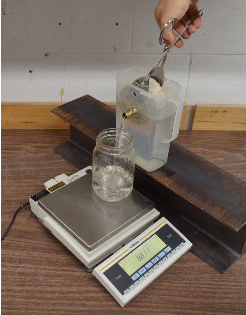
Figure J.1 Determination of volume by displacement.
