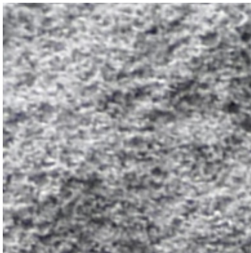
Figure 7.3.3j Horizontal fracture surface was filled with debris for 410kg/m 3 cem. dens., 0:1 filler-binder ratio mix. 4x magnification
