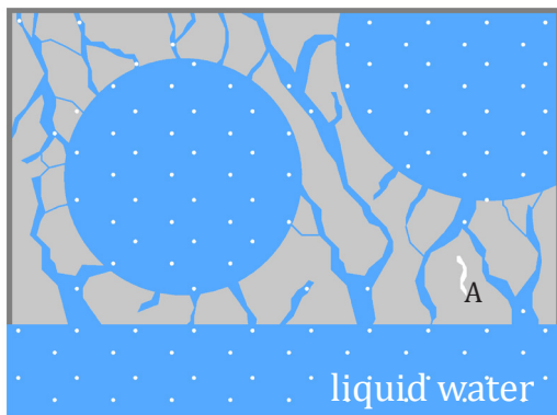
Figure 7.3.7f Vacuum Saturation Specimen dried, then vacuum saturated.
