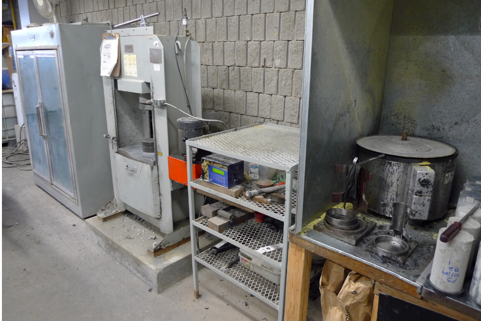
Figure 5.4.1a Specimens were capped with sulphur and tested for compressive strength.
