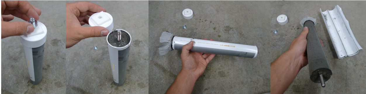
Figure 5.1.4c Demoulding process for 50 x 300mm diameter specimens, used for drying shrinkage testing. Refer to Section 5.5.1.
