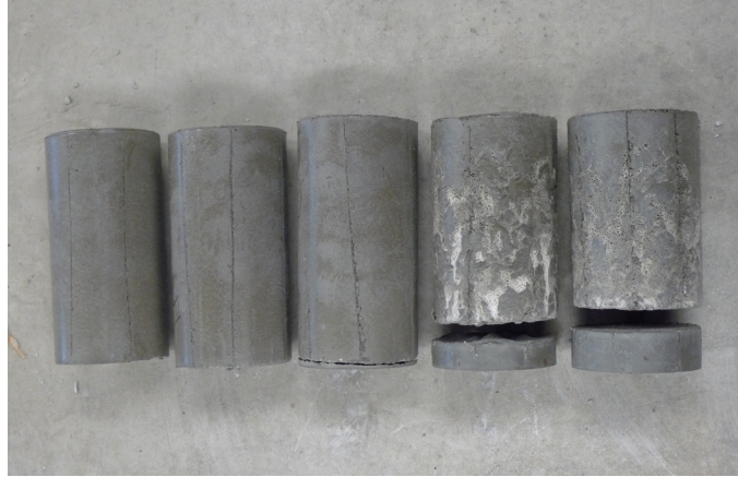
Figure 6.1.1b From left to right, water-binder ratios of 0.6, 0.65, 0.7, 0.75, and 0.8. Segregation is evident in mixes with high w/b ratios. Note the whitish veins running through specimens on the right, where cement has dropped from the mix.
