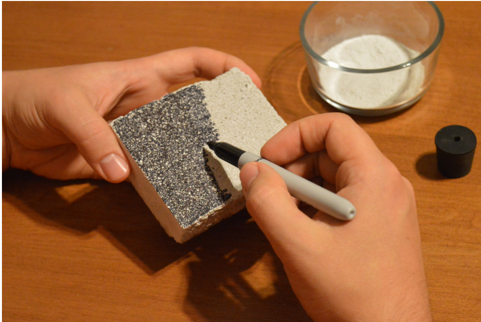
Figure 5.8.2a Surface of specimen coloured in black for air-void analysis.
