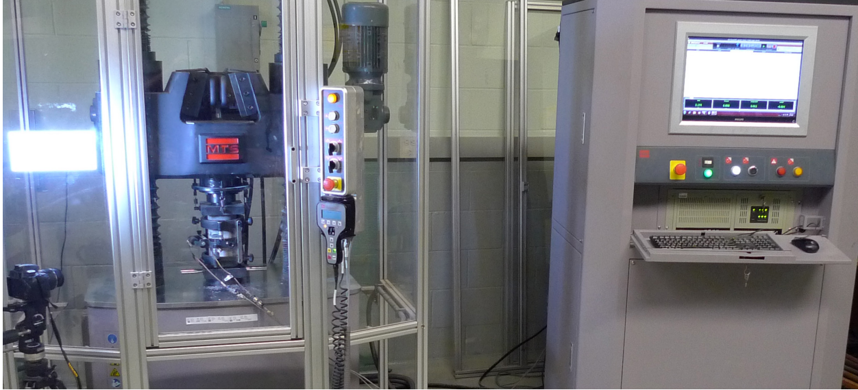
Figure 5.4.2a Set-up for testing of modulus of elasticity and Poisson's ratio. An unbonded compressometer is attached to the specimen; the specimen is seated centrally in the testing frame. As load is applied, changes in specimen height and diameter are recorded continuously.
