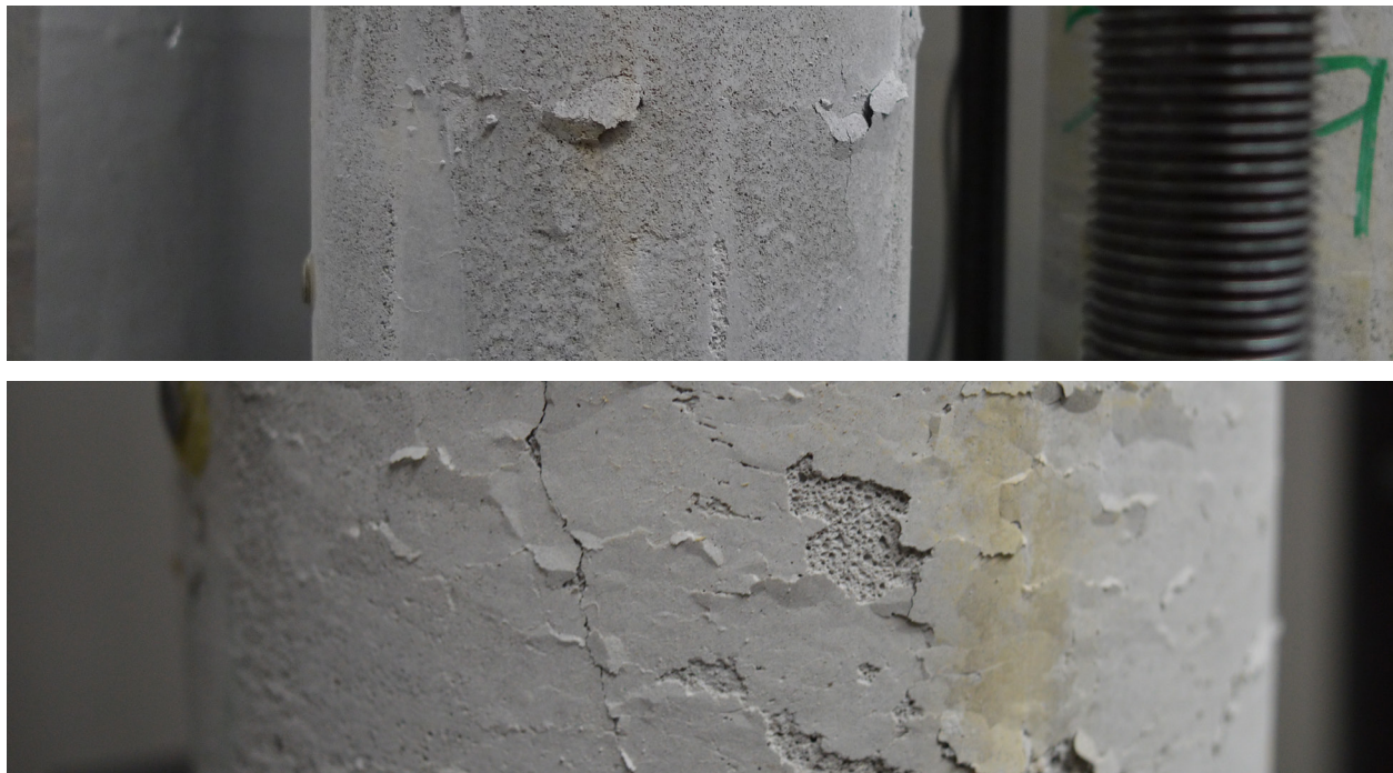
Figure 6.10d Buckling along cast surface of 600kg/m 3 foam concrete after 12 months of exposure to 50% RH, for loadings of 0.2 and 0.4 f'_c (above and below, respectively).
