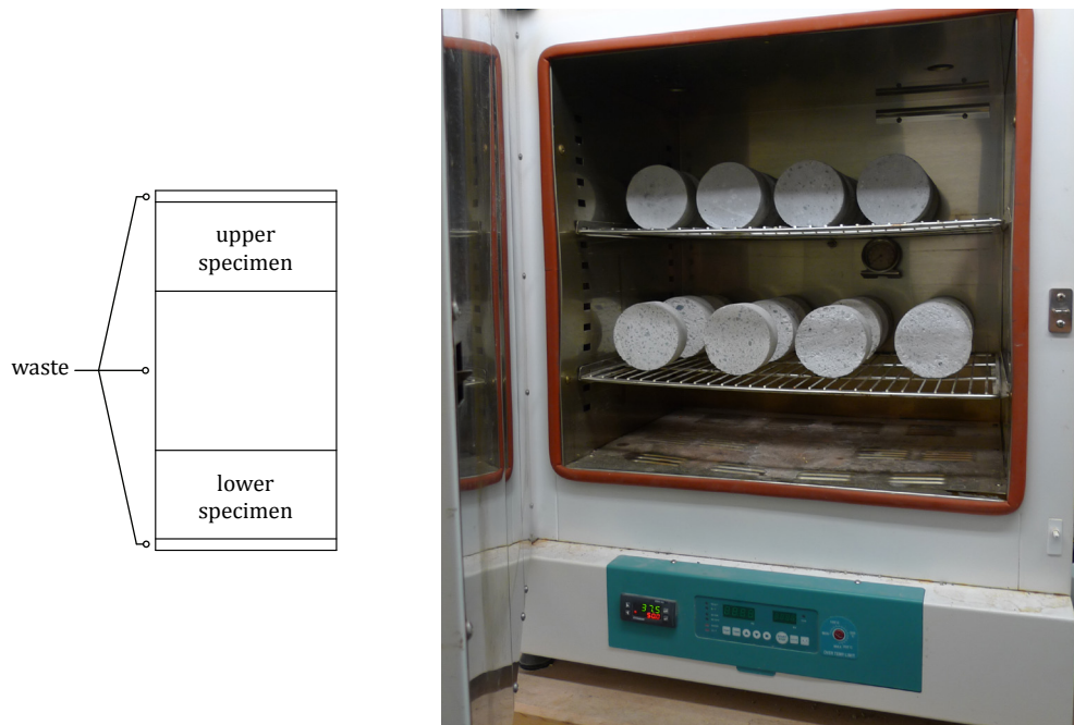
Figure 5.3.2 50mm high specimens were cut from the bottom and top of 100 x 200mm cylinders for segregation testing (left), and oven-dried (right). A 6mm thick layer was removed from the top and bottom surface of the cylinder, to eliminate local effects of particle packing and finishing on density.
