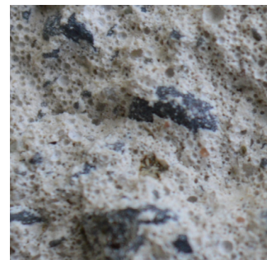
Figure 7.3.3l Diagonal fracture surface was highly irregular for 410kg/m 3 cem. dens., 3:1 filler-binder ratio mix. 4x magnification
