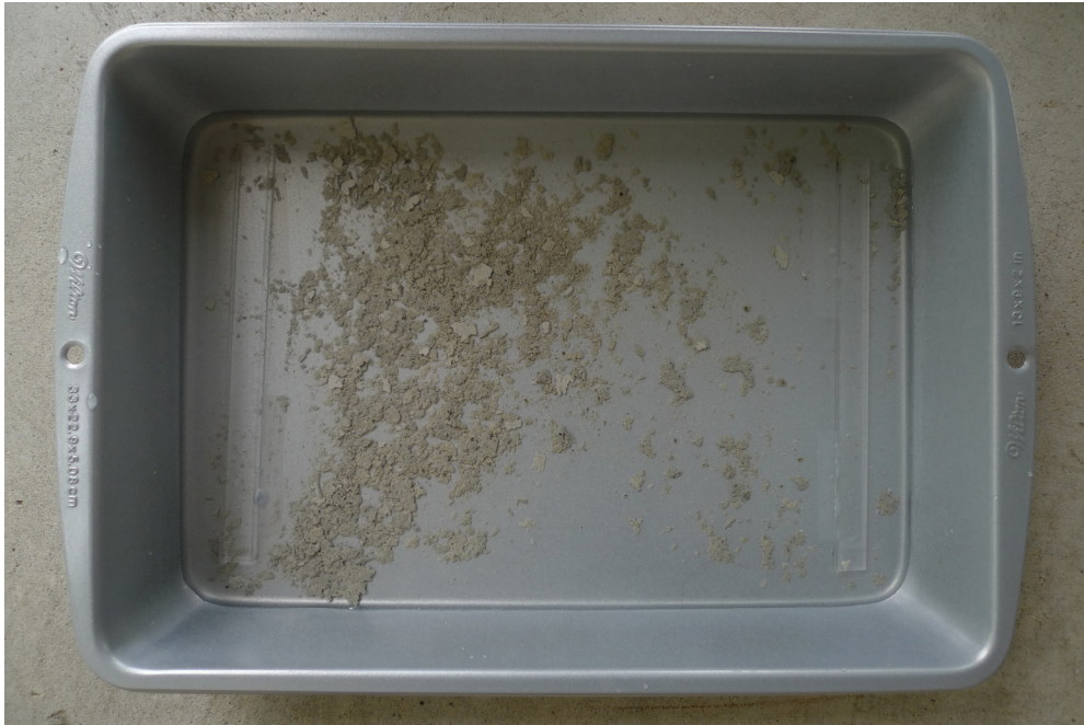
Figure 5.7.2b Typical accumulation of loose flakes and particles of concrete (scale) from foam concrete panel surface after 5 freeze-thaw cycles in 3% sodium chloride solution. Images of scaled surfaces are shown in Section 6.16.2.
