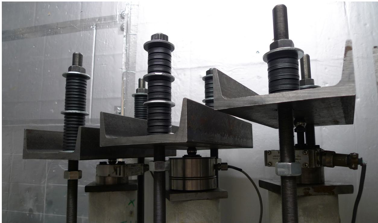
Figure 5.4.5b Detail of creep frames. Specimens bear against thick steel platens. Load cells bear against spherical steel spheres, centred in conical depressions in the steel frame, to reduce eccentric loading on the cylinder stack. Varying combinations of disc springs, tuned for each intended load, reduce variation in applied loading as the specimens deform. Nuts on the threaded rods are tightened regularly to accommodate displacement.
