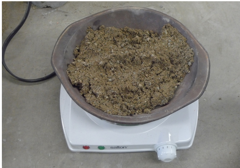
Figure D.2.1 Sample of sand dried on hot plate to determine moisture content.
