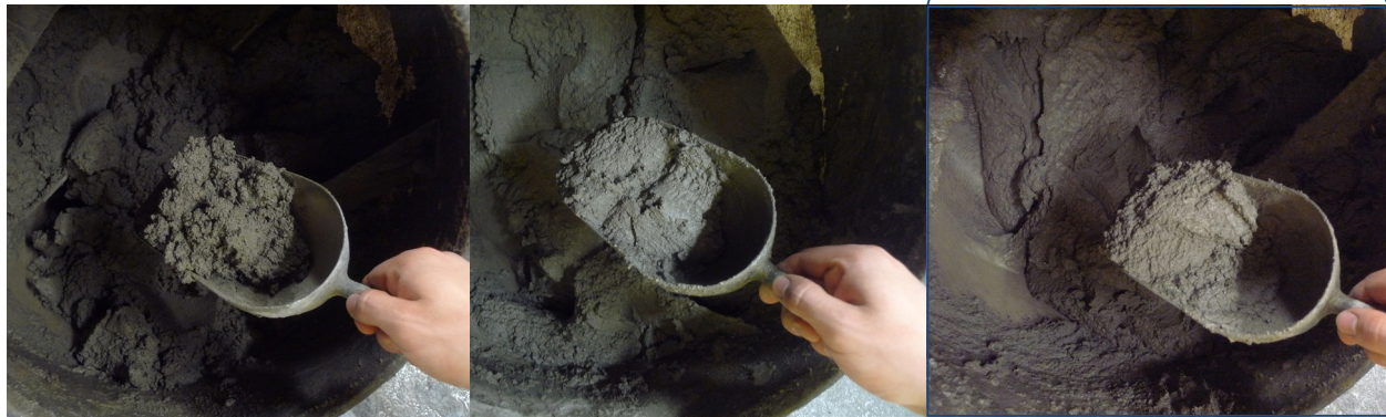
3:1 filler-binder ratio, 0% foam (base mix) 3:1 filler-binder ratio, 7% foam by volume 3:1 filler-binder ratio, 15% foam by volume
