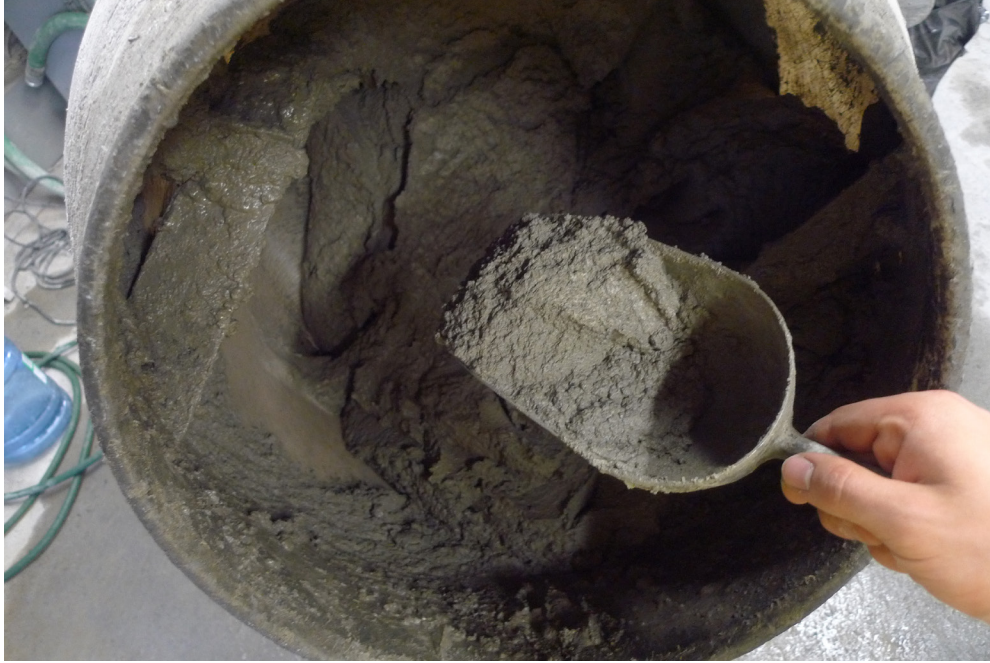
Figure 5.1.3a Image of thoroughly blended, fresh foam concrete in a laboratory mixer.
