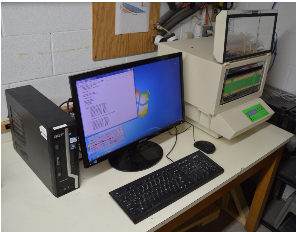
Figure 5.6.1b Set-up for thermal conductivity testing. Specimen is loaded in the guarded hot plate apparatus on right. Heat transfer between the hot plate, panel, and cold plate is automatically recorded every minute until steady state conditions are achieved.
