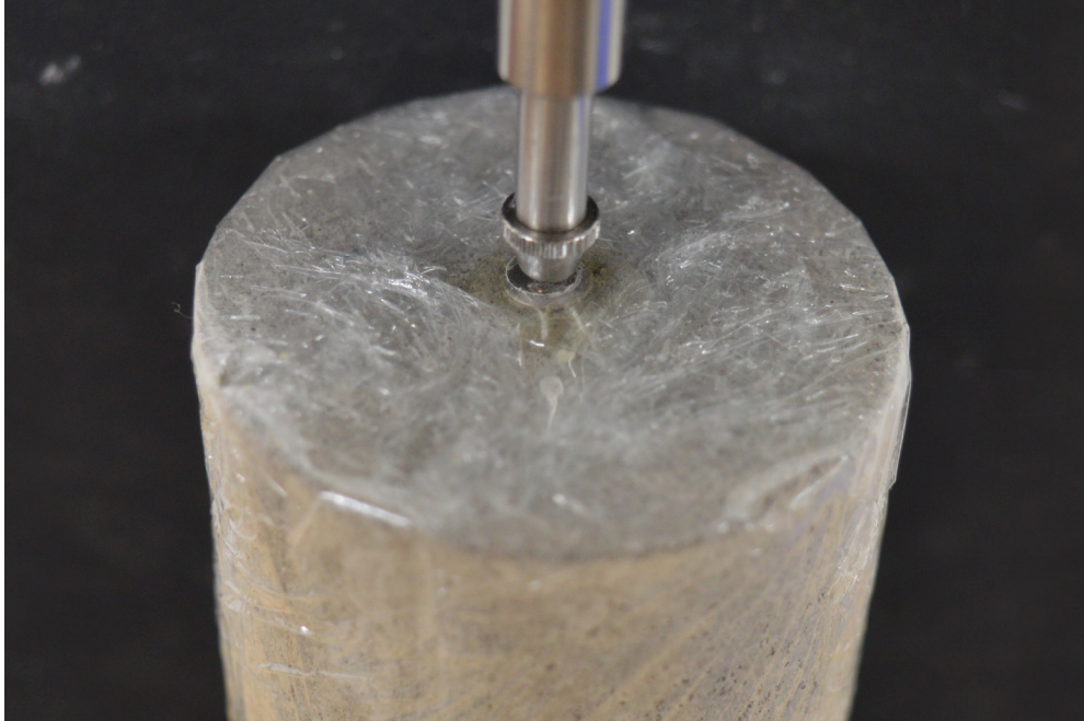
Figure 5.7.1a 50 x 150mm specimen sealed to prevent moisture loss. A 4mm diameter aperture in the taped ends, centred on the stainless steel locating discs, facilitated a positive connection to the terminals of the length comparator.
