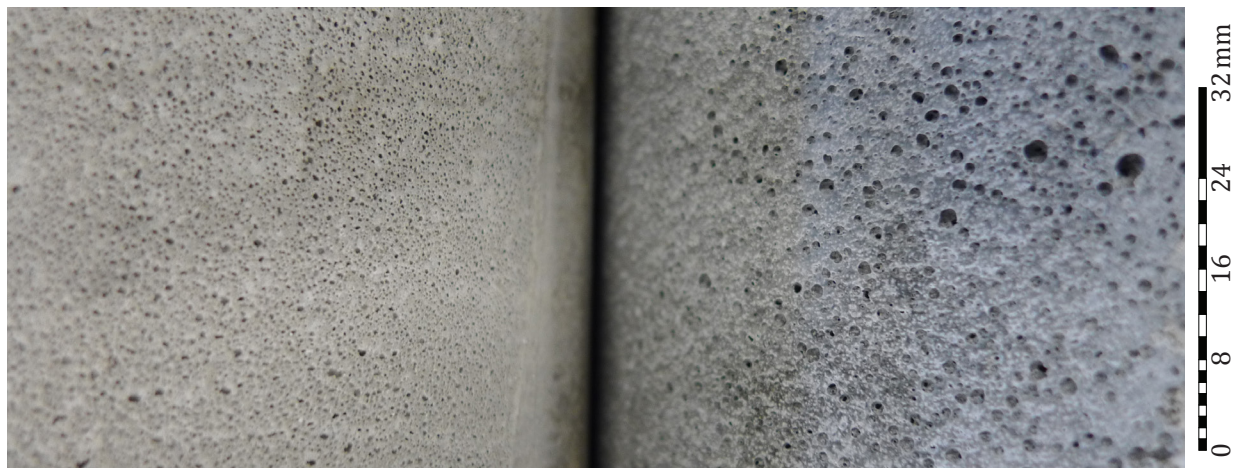
Figure P.1 Comparison of the cast surfaces of conventional (left) and superplasticizer (right) mixes. Note the coalescence in the superplasticizer mix. The closest portions of cylinders are at 1.5x magnification.
