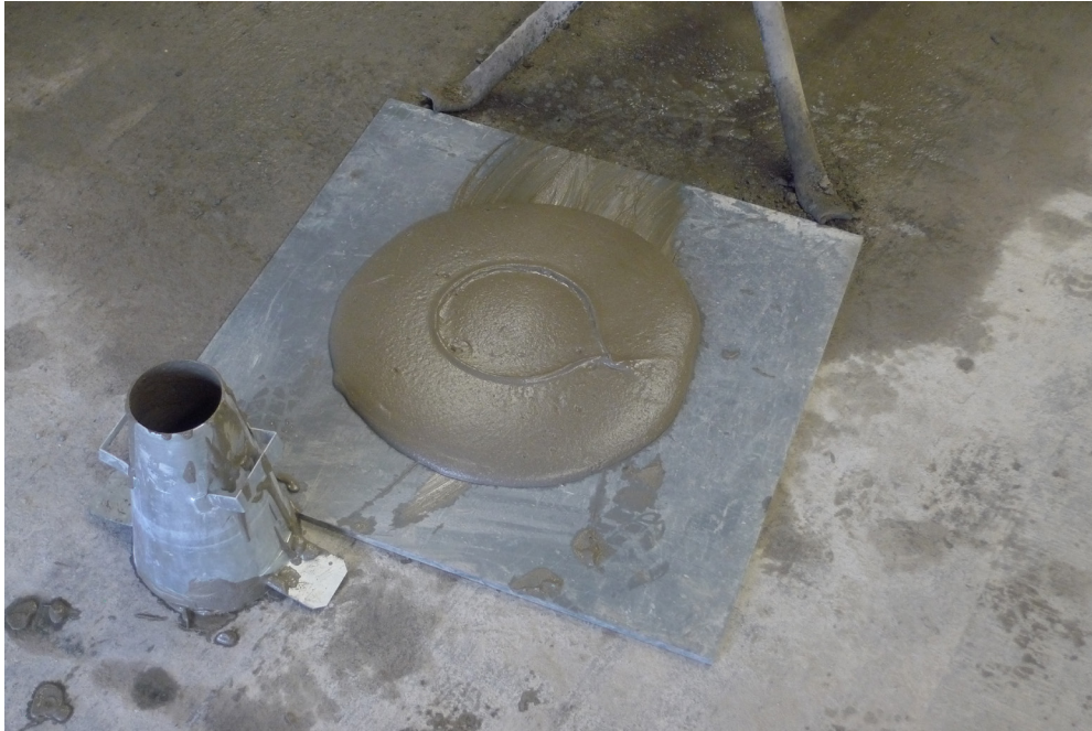
Figure 5.3.1 Typical spread of fresh foam concrete.
