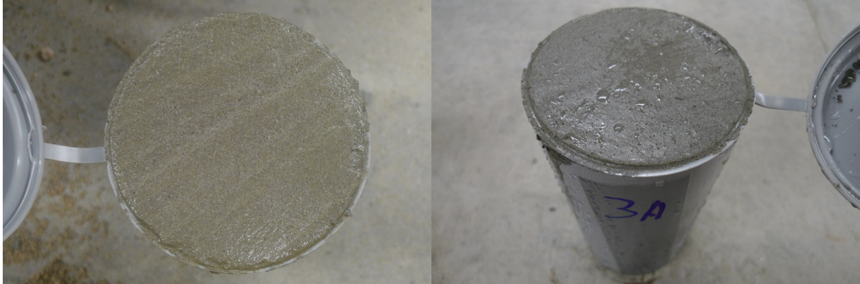
Figure 5.1.4a Typical finished surface of fresh (left) and hardened (right) foam concrete in 100 x 200mm plastic moulds. The mix on the left is sanded, while the mix on the right contains no aggregate.
