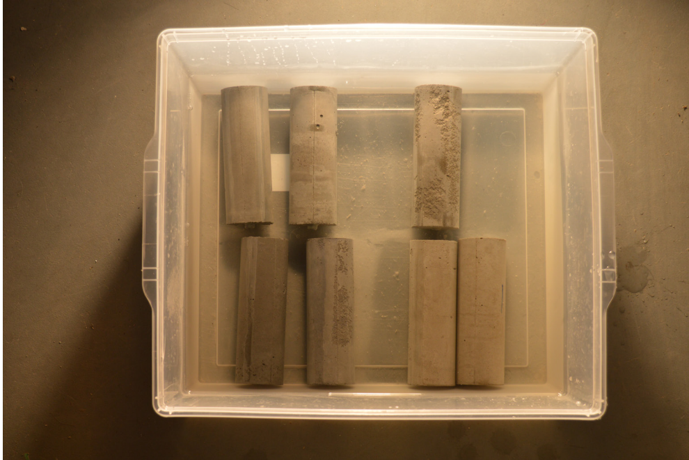
Figure 5.5.4a 50 x 150mm specimens immersed fully in water, for water absorption and moisture movement testing.
