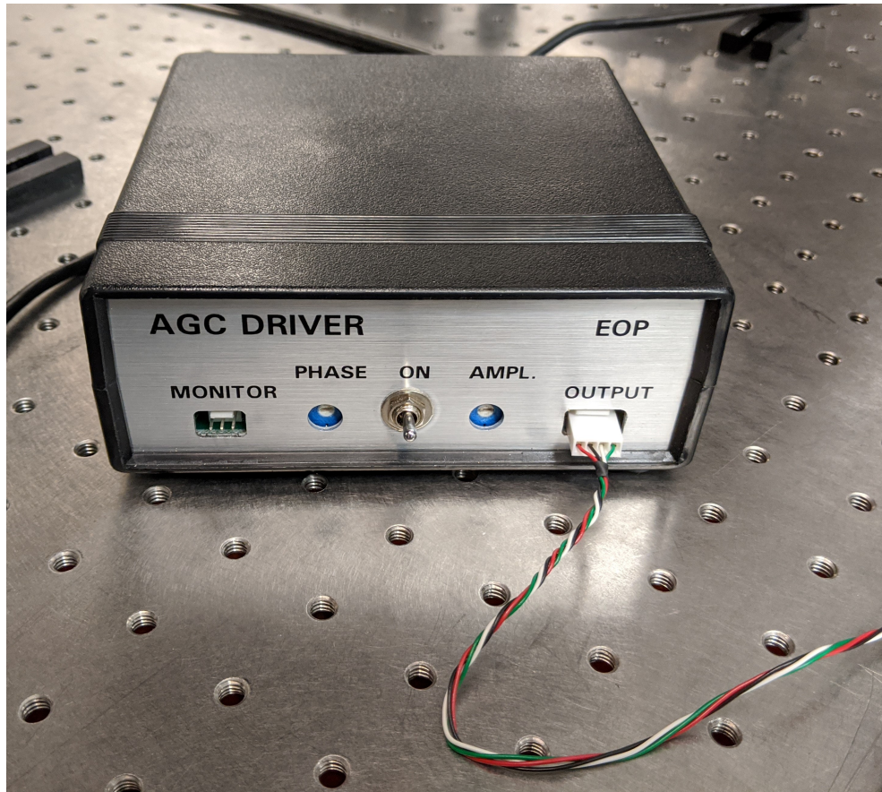
Figure E.2: Photo of the AGC driver and its phase and amplitude tuning knobs.
