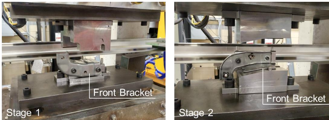
Figure 210. Reforming of the production front bracket broken down into two stages: Stage 1 (left) the bracket face is reformed to match the enclosure panels inner face, Stage 2 (right) fold initiator is formed into the bracket.
