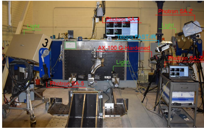
Figure 76. Arrangement of high speed cameras and lighting around the specimen for the eighth baseline front end module test (Bd-9).
