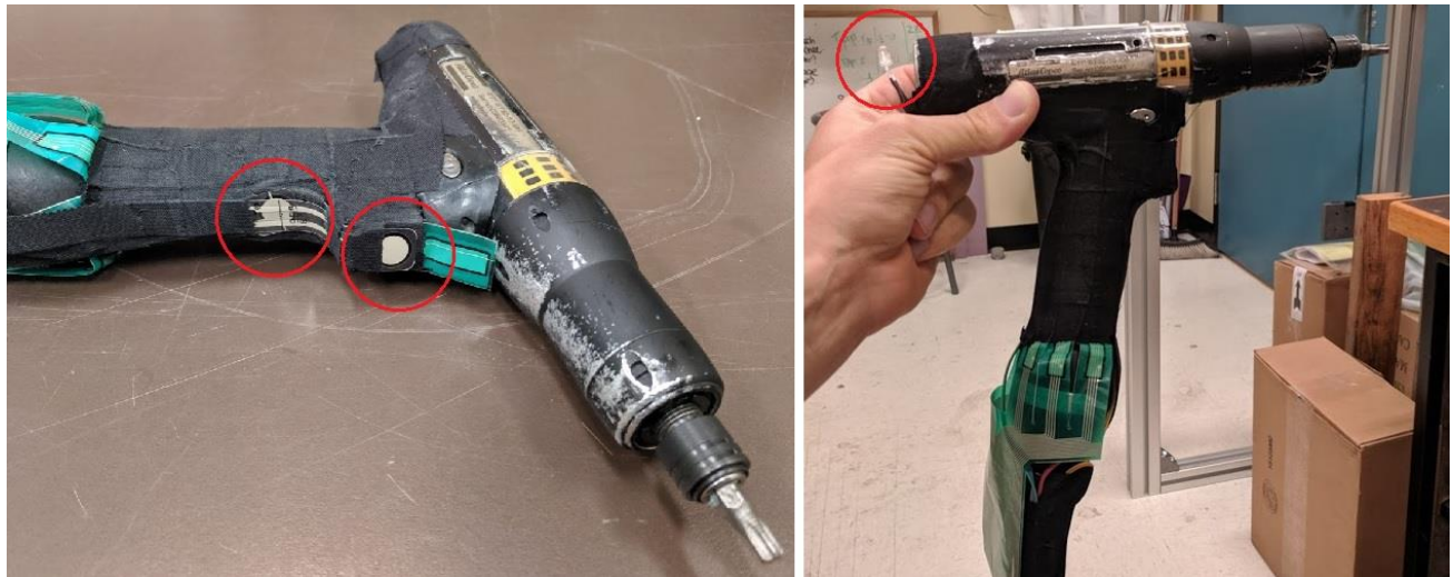
Figure 40 Grip trainer FlexiForce sensors (left) and visual feedback LED placement (right) on the tool
