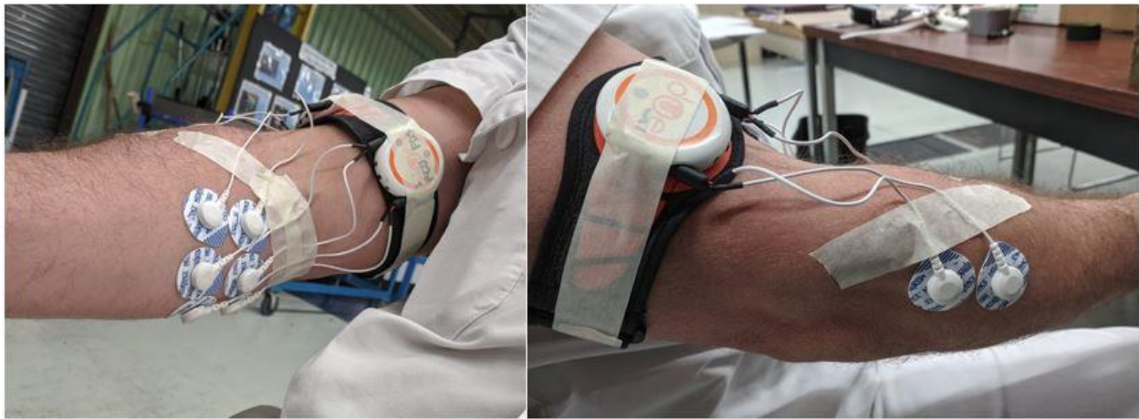
Figure 38 Example of EMG electrode and probe placement for FCU, FDS, FCR (left) and EDC (right)
