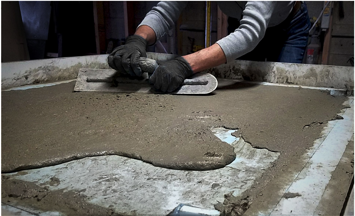
fig. 20 Trowelling the mix as thin as possible to reduce weight on the underside of a coffee table
