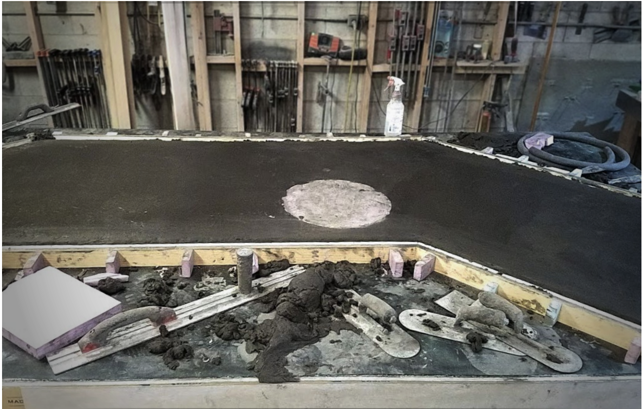
fig. 13 Chaotic aftermath of a struggle with the timing of a countertop cast
