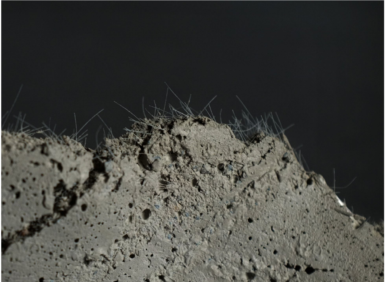
fig. 7 Broken ECC with fibers exposed
