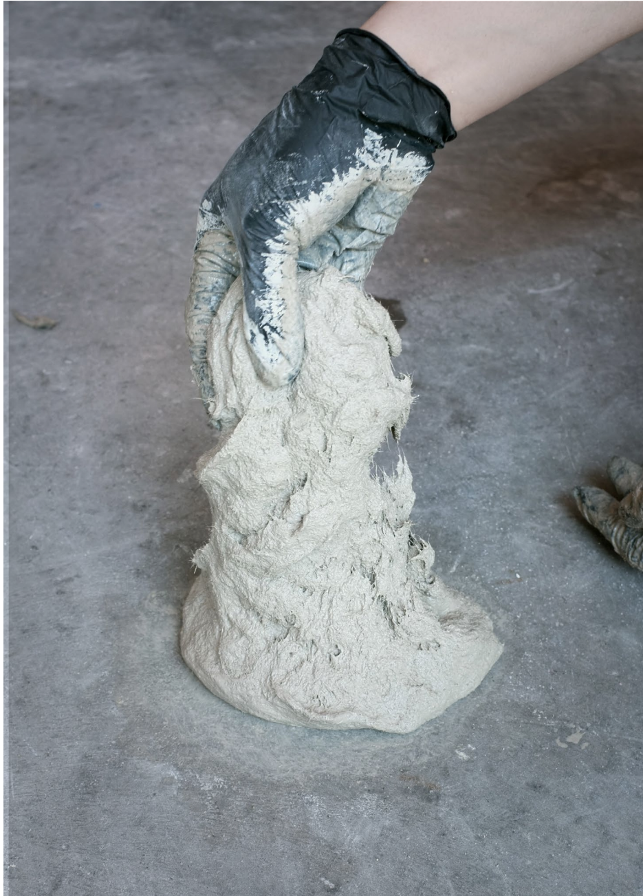
fig. 10 Plastic phase of ECC
