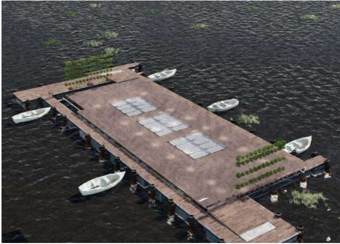
FIGURE 4.22 1st floor showing the floating docks, Fish tank platforms and wooden floor panels
