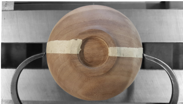
fig. 2.13 Measuring the Diameter
