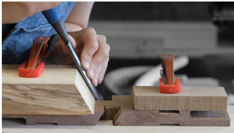
fig. 3.62 Chiseling the Three-Way Lap Joint with a Jig
