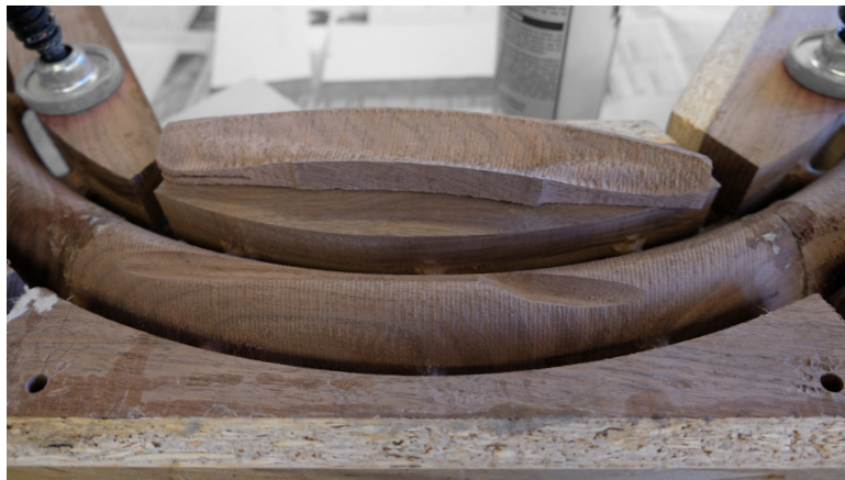
fig. 3.37 Backrest Plug and Gouge
