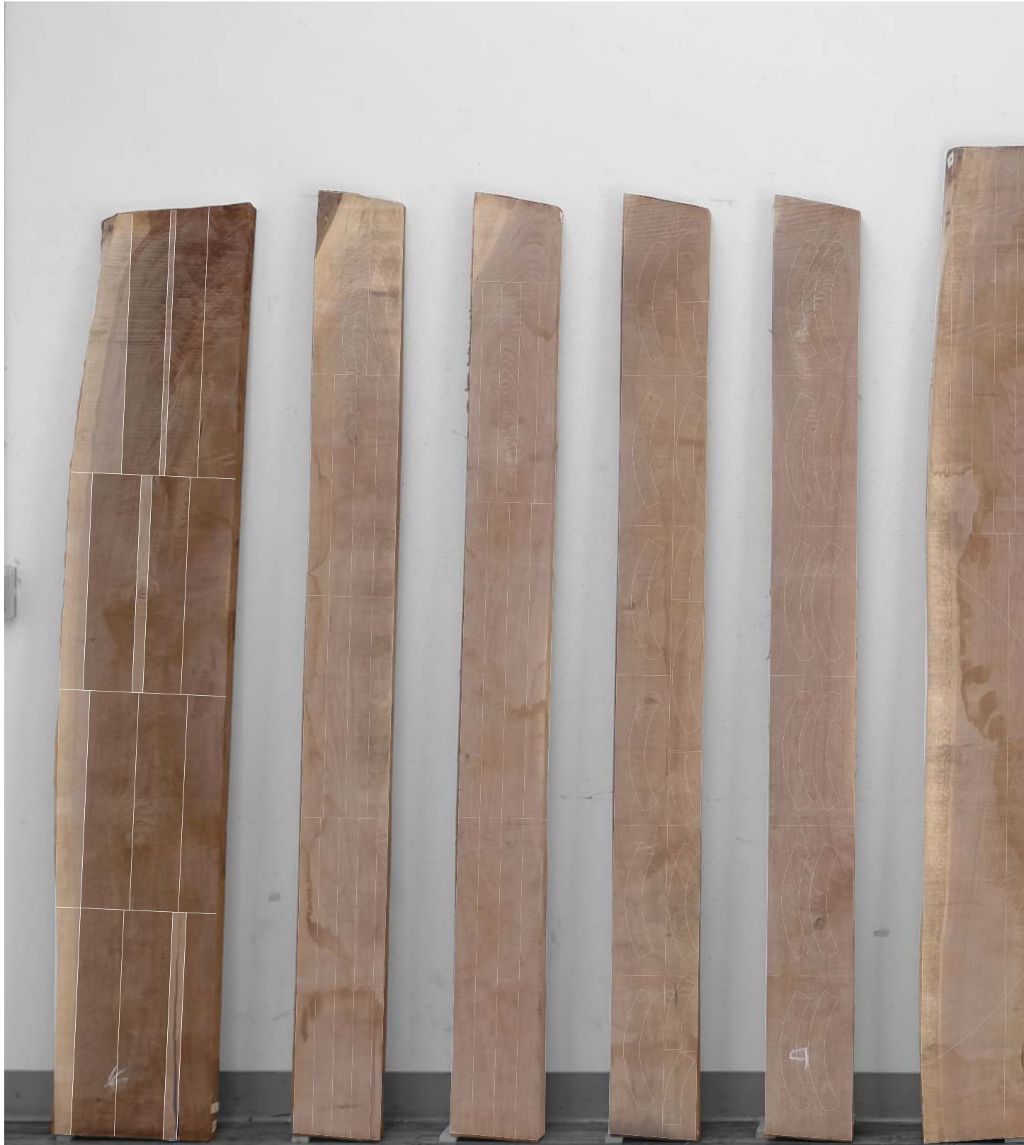
fig. 5.4 Chair Seat Rough Cut Diagram
