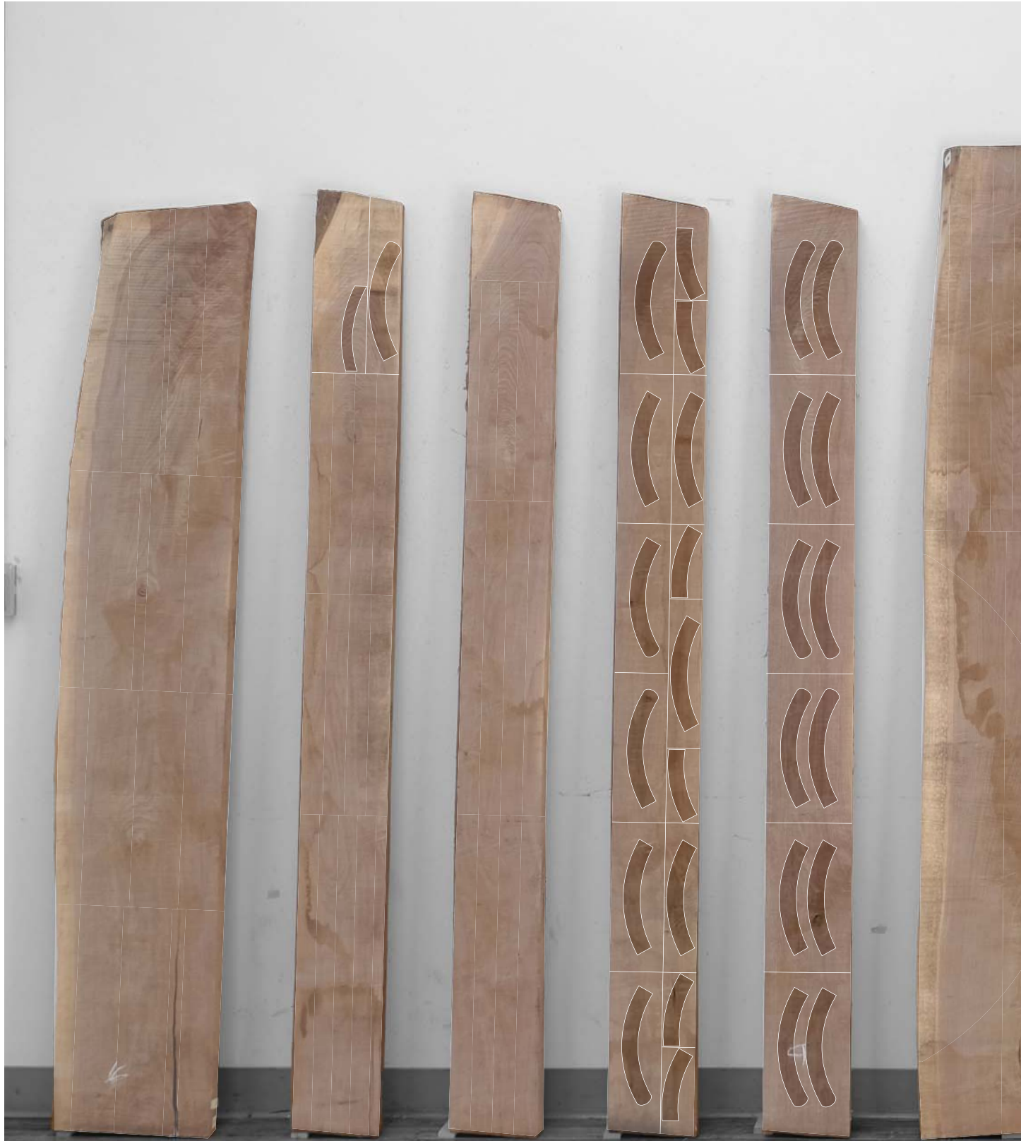
fig. 5.6 Chair Back Rough Cut Diagram
