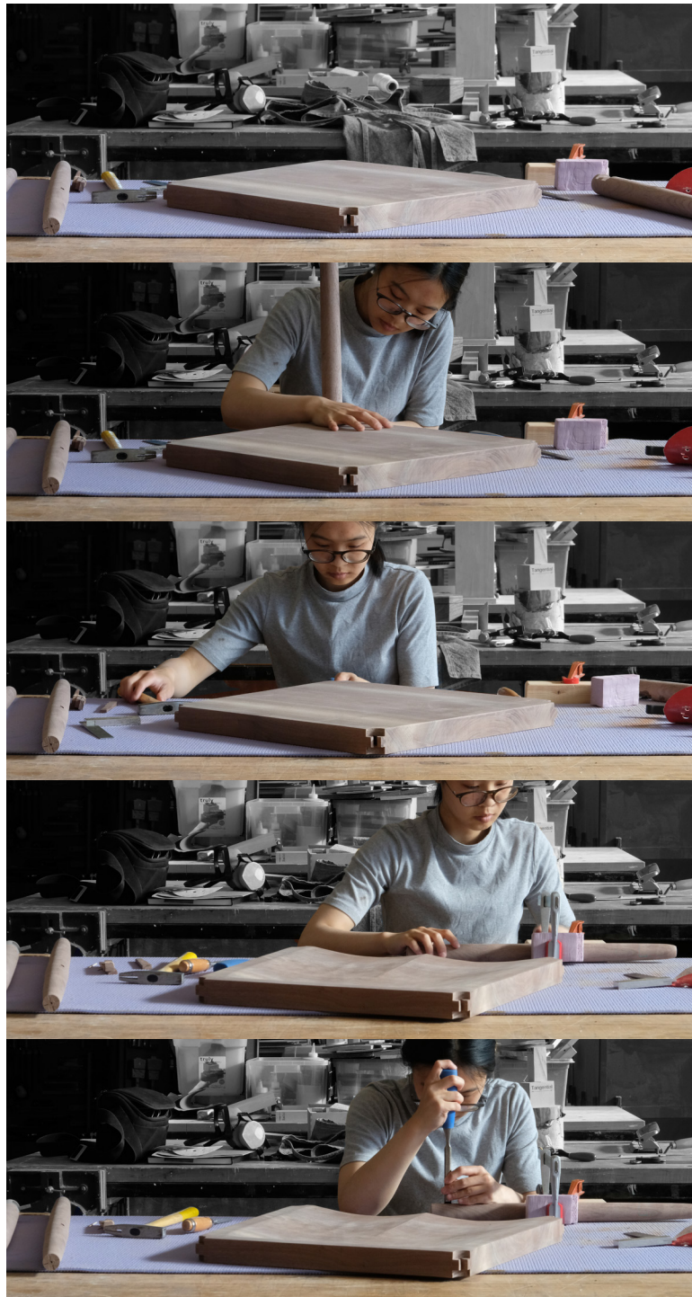
fig. 3.17 Fitting the Chair Joints
