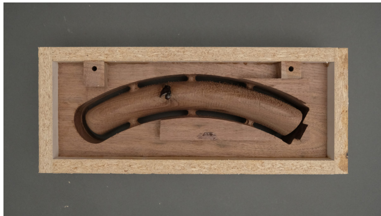
fig. 3.38 Right Backrest Arm After Milling
