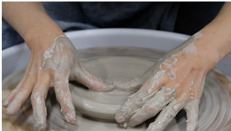
fig. 2.32 Flattening the Plate
