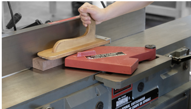
fig. 2.16 Jointing a Face
