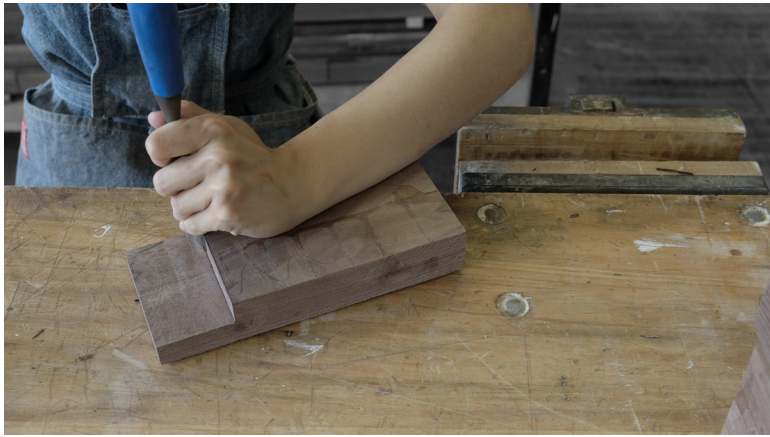
fig. 3.58 Chiseling Lap Joints
