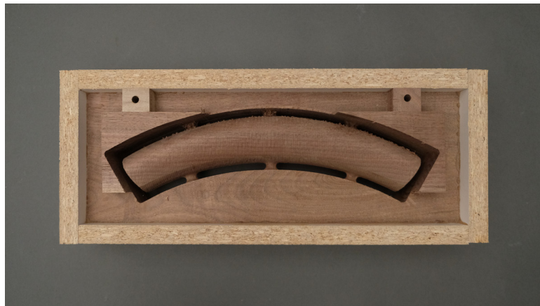
fig. 3.40 Middle Backrest Part After Milling
