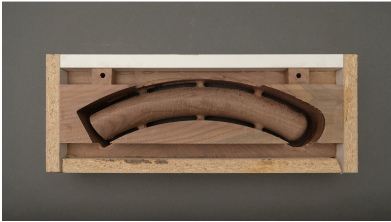
fig. 3.42 Left Backrest Arm After Milling
