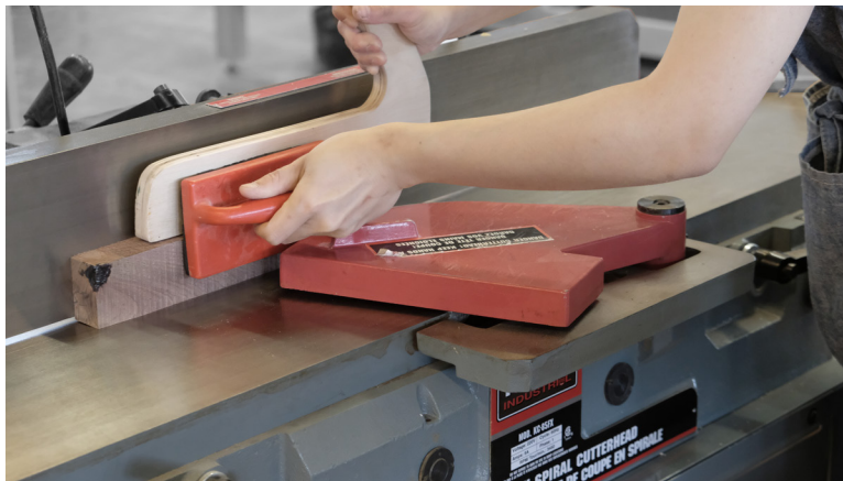
fig. 2.17 Jointing an Edge
