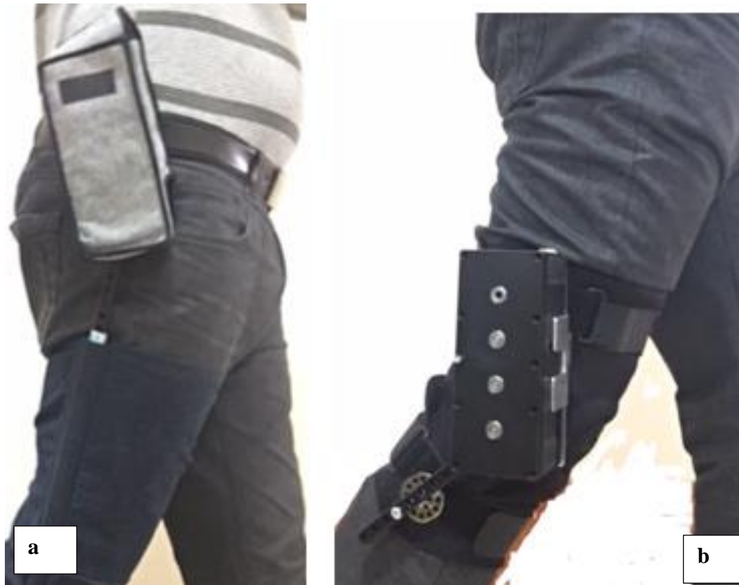
Fig. 4.17 - Typical Human Interface – (a) Hip-mounted installation on the left and (b) Knee-mounted installation on the right.
