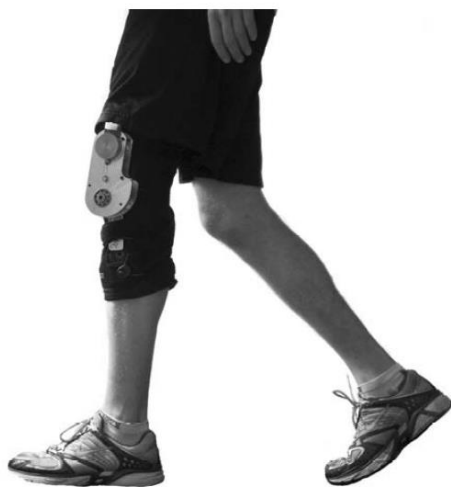
Fig. 2. 2 - The biomechanical energy harvester comprises an aluminum chassis and generator (cylindrical component at the top of the chassis) mounted on a customized knee brace (black) [18].
