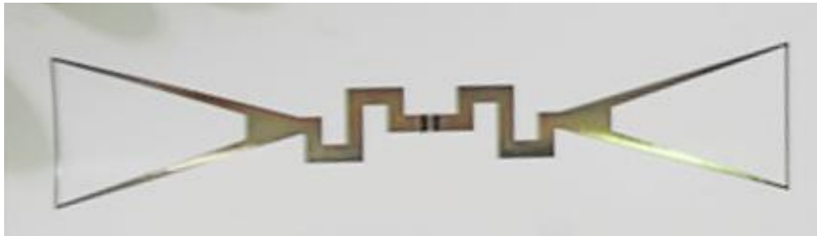
Fig. 2. 11 - RF Energy Harvesting Sensor node printed on paper using inkjet technology [39]
