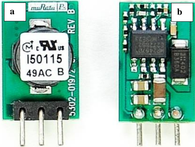
Fig. 4.13 – OKI-78SR DC-DC converter (a) front side (b) opposite side
