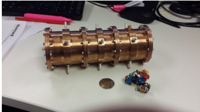
Figure 6.2.4.4. Manufactured triple-band filter with elliptical cavity.
