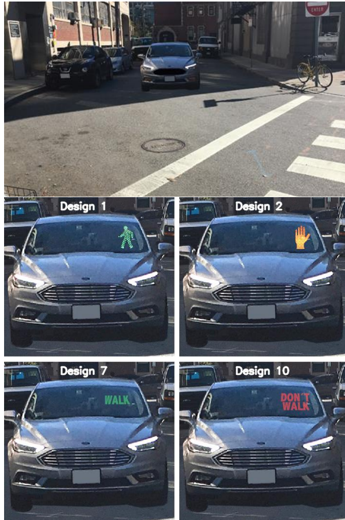
Figure 3. Most effective designs found in terms of perceived safety from Fridman et al., 2017
