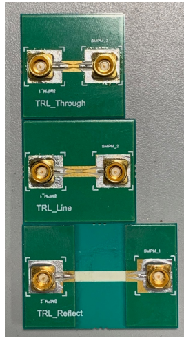
Figure 5.1: Designed TRL calibration kit
