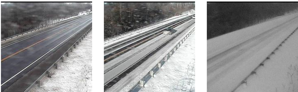
Figure 1.1: Example images from a roadside camera near Otter lake in Ontario. Left: Bare pavement. Center: Partial snow cover. Right: Full snow cover.
