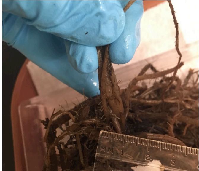
Figure 2.14: Photo illustrates the determination of the number of roots within 1 cm 2 from a Typha root ball. This method was also used to determine the root density root parameter.
