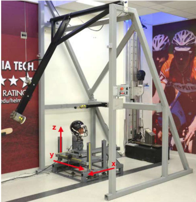
Figure 2.10 (a) Virginia Tech pendulum impactor and sliding carriage [15]
