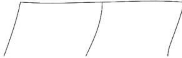
Figure 10 – Buckled shapes of frames in Scenario 13 (worst case delamination in Column 3)
