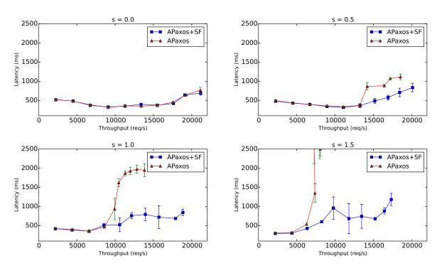
Figure 7.1: Latency vs throughput for 5 replicas under different levels of skewness of client load.
