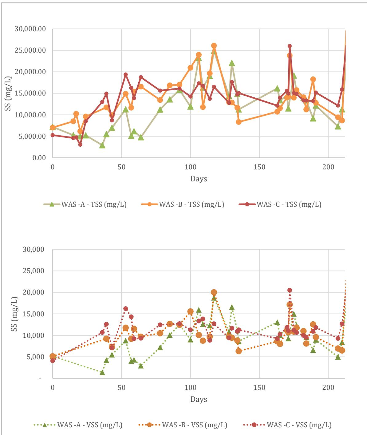
Figure 4. 8: Suspended Solids for All three reactors in phase 1
