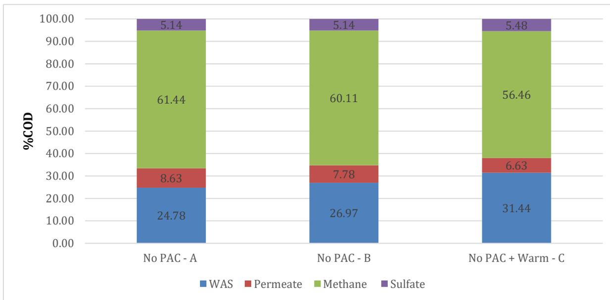
Figure 4. 11: COD distribution in the three reactors during phase 1
