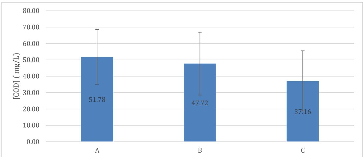
Figure 4. 10: The Average and standard deviation of permeate quality in all three reactors
