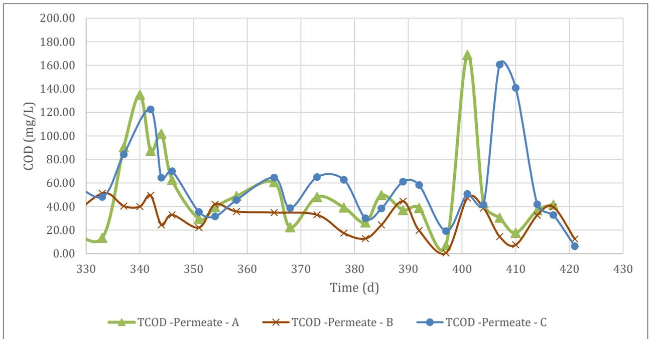
Figure 4.19: COD in permeate samples for reactors I phase 2
