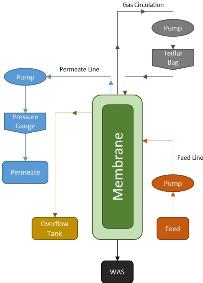
Figure 3. 2: Experimental Configuration
