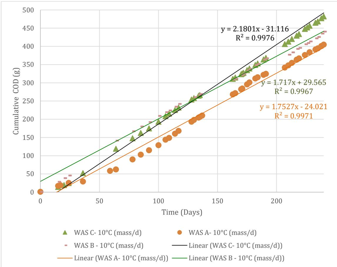
Figure 4. 6: Cumulative TCOD in WAS in phase 1 for all three reactors
