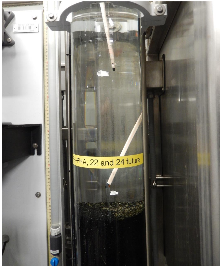
Figure 3-7. The deep bed filter in Toronto R.C. Harris Water Treatment pilot plant during ripening experiment. Tubing with a small rod attached to: fit through metal grate half way down the filter column, and be closer to the filter bed to shorten the oocyst travel time and capture the 30 minute ripening period.
