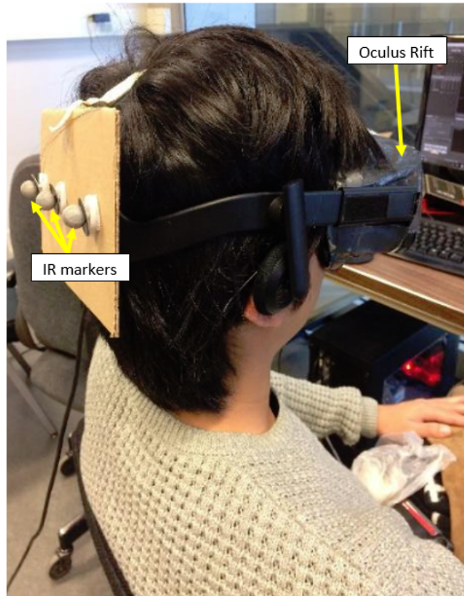
Figure 3.1: Oculus Rift with IR Markers.
