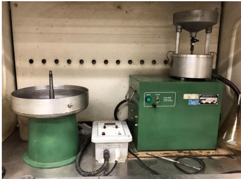
Figure 29 Centrifuge Extraction Apparatus
