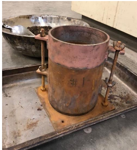
Figure 38 CBR Test Compacted Mold
