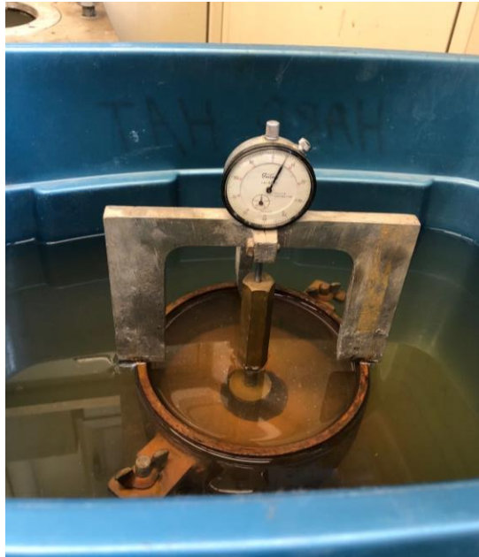
Figure 39 CBR Soaking Test
