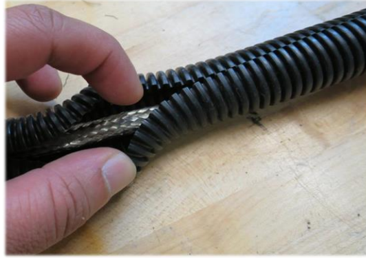
Figure 5.41: LV EMI Shielding
