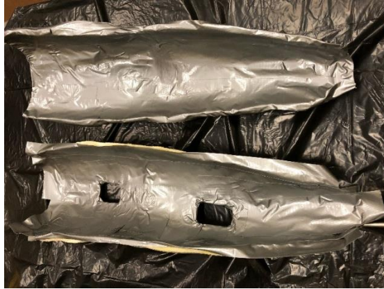
Figure 4.13 The inside of the cast lined with duct tape to prevent it from sticking to the foam mould
