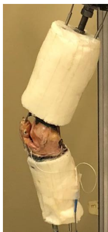
Figure 4.15 Medial sagittal plane view of a leg covered in foam with the foam and carpet cut away from the knee joint
