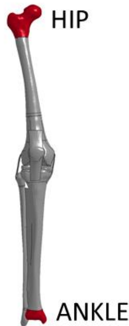
Figure 6.11 End caps for application of hip and ankle boundary conditions - anterior frontal plane view
