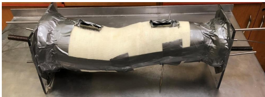
Figure 4.14 The sealed cast oriented using the end plates ready for the foam to be poured
