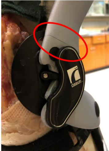
Figure 5.3 Crack in the knee brace of knee 1
