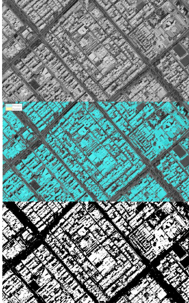
Figure 6.3 (a)Pre-processing, (b)threshold adaptation, and (c)post-processing images depicting the rooftop area of buildings in the sample region
