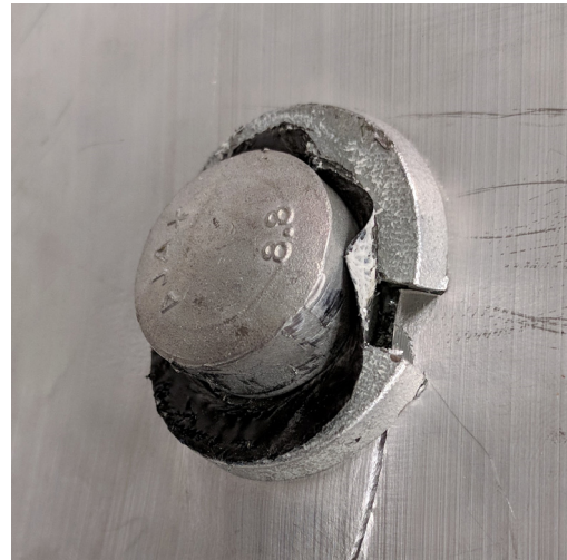
Figure 6.9: Separation of folded stepped washer
