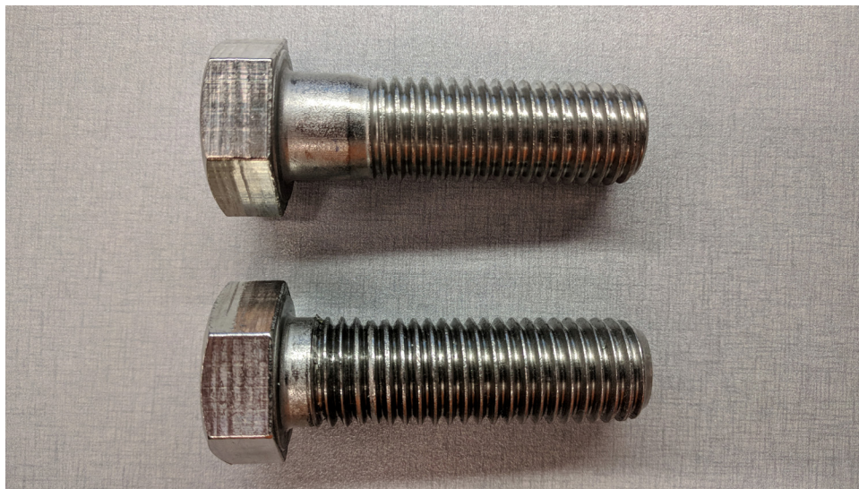
Figure 5.3: \frac{3}{4} " stainless steel bolt with unmodified threads (top) and extended threads (bottom)
