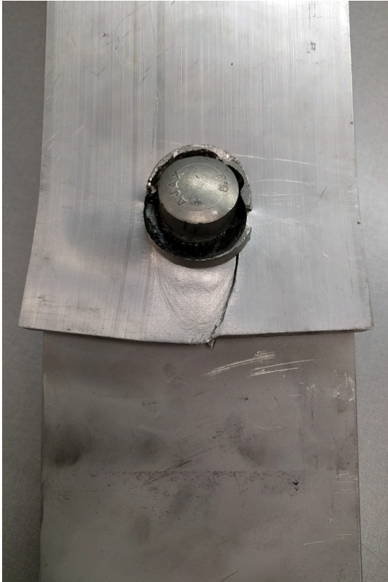
Figure 6.2: Block shear failure of Specimen FSBS1-S
