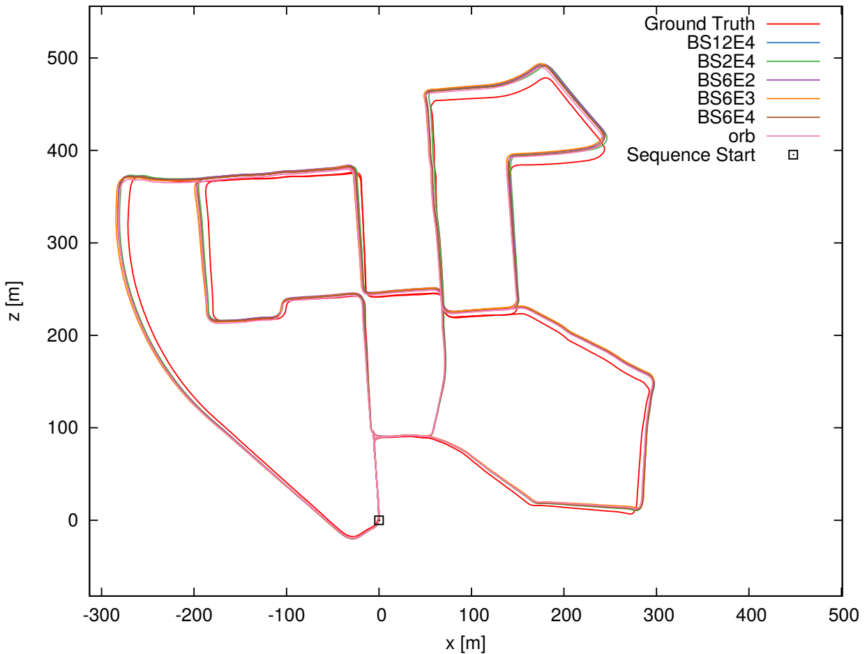
Figure 4.7: Overlaid trajectory results for sequence 00 from the KITTI odometry set comparing various SIVO configurations, ORB_SLAM2, as well as the ground truth.
