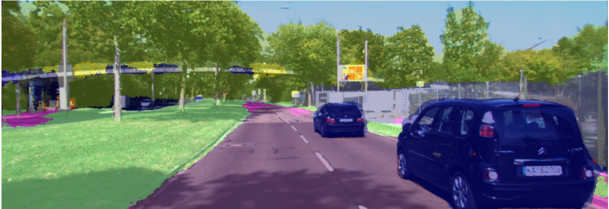
(a) Semantic segmentation results from the KITTI semantic validation set. This result is the average of 40 stochastic passes of MC dropout.
