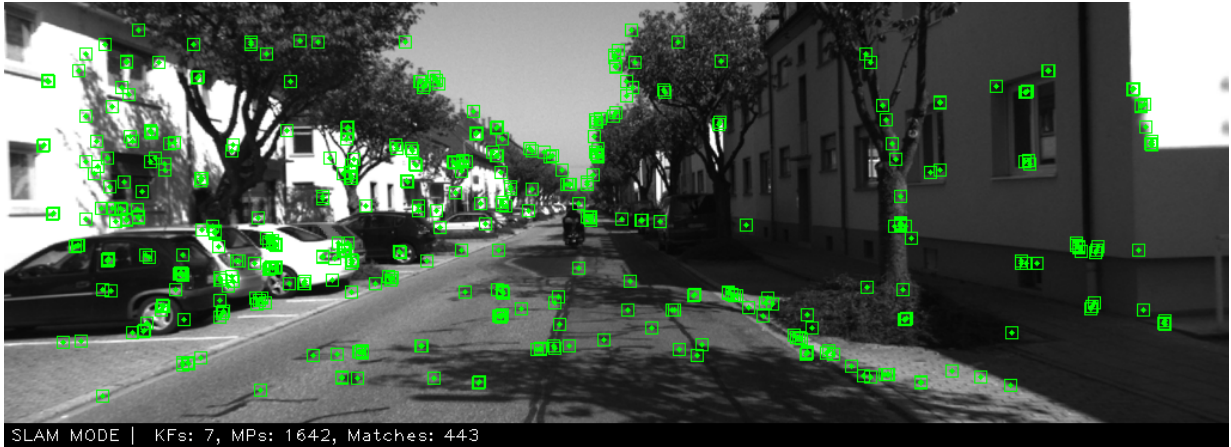
(a) ORB_SLAM2 extracting features on KITTI sequence 00. There are a number of stationary cars which ORB_SLAM2 uses for localization. These points are excellent for short-term localization, but are poor for long-term map construction.
