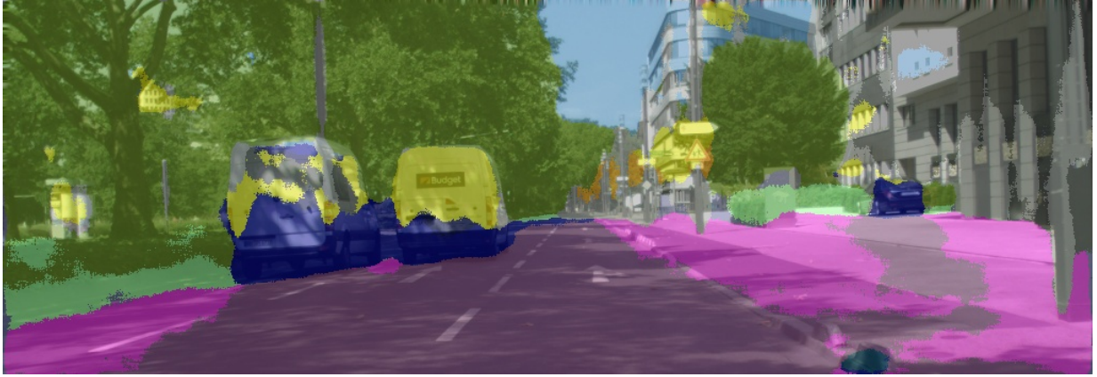
Figure 3.1: Example of low quality image segmentation. In this scenario, the logo on the right van (blue) is being misclassified as a traffic sign (yellow), while the left van is being misclassified as a building (grey).
