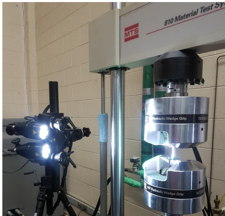
Figure 20. Quasi-static tension test setup.
