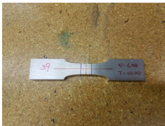
Figure 30. Smooth cyclic test sample (the marked blue lines are where the extensometer knife edges are contacting the specimen)
